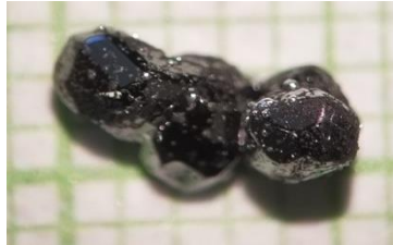
Figure A3.1: Image of typical crystals of \text{Yb}_{14}\text{MnSb}_{11} grown from Sn flux and employed in this study. Droplets of Sn flux can be seen on the surface of the crystals.
