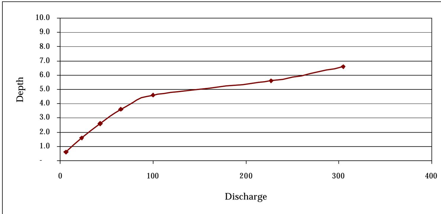
*Note: This rating curve illustrates the average depth/discharge relation among the two cross-sections analyzed.*
