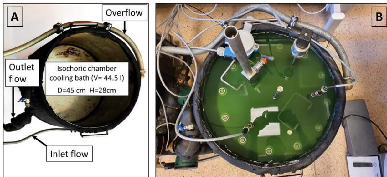
Figure 6. (A) Isochoric chamber cooling bath. (B) Isochoric chamber immersed in the cooling bath fluid.
