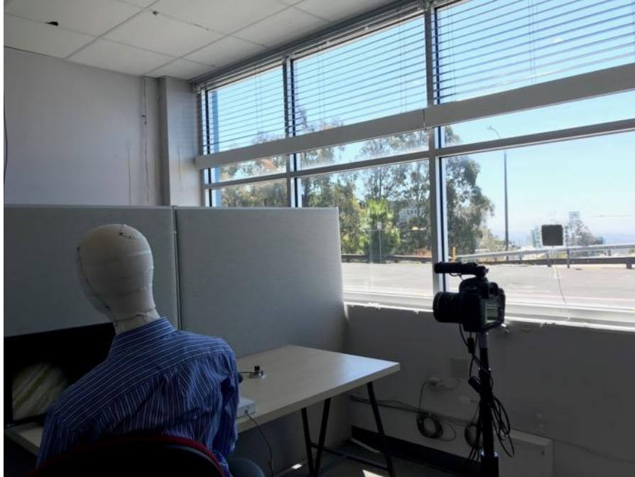
Figure 10. Photo of HDR camera and sensor positioned for glare analysis in FLEXLAB
