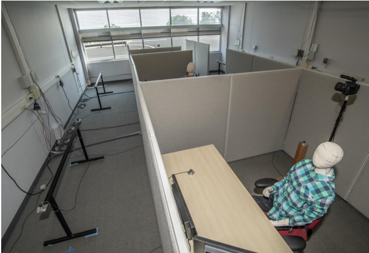
Figure 7. Photograph of retrofit cell layout. Automated blinds are set to a neutral angle ( 0^\circ ) and automated rollershades are deployed at a length of approximately 10 inches.
