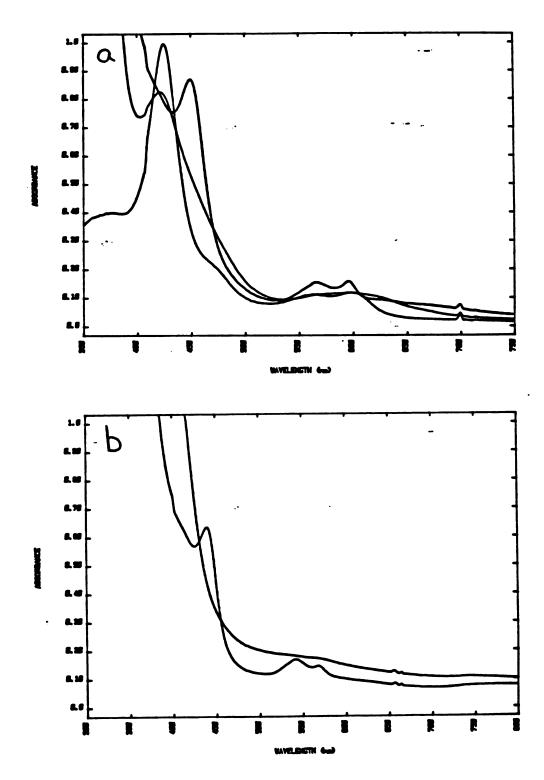
Purified P-450cam was incubated with (a) diazoacetophenone or (b) ethyldiazoacetate and then reduced with  $Na_2S_2O_4$  to form the 445 nm complexes. The spectra in (a) show the native P-450 Soret band at 418 nm, the reduced P-450, and the fully formed complex at 445 nm.
