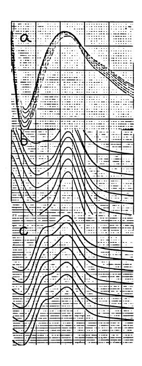
The Electronic Absorption Spectra of incubations of microsomal P-450, NADPH and (a) Ethyldiazoacetate, (b) Diazoacetophenone, and (c) 1-diazo-1-phenyl-2-propanone. The series of spectra are repeated scans during a 10 minute period.
