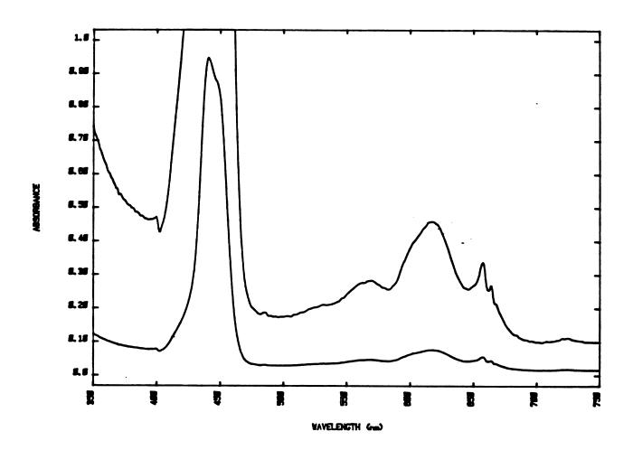
The zinc complex of the TPP-DAP adduct was prepared by adding  ${\rm Zn}\left({\rm OAc}\right)_2$  to a solution of the porphyrin. The resulting bluegreen complex has a soret maximum at 435 nm.
