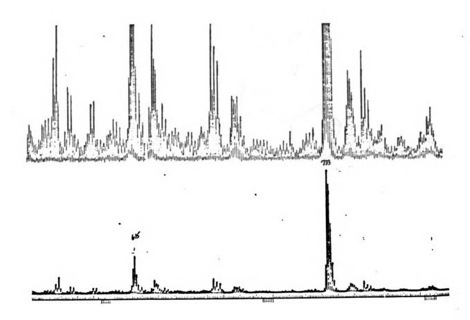
The TPP-DAP complex was demetallated over night with 5%  $H_2SO_4$ /methanol and analysed by LSIMS mass spectrometry in sulfolane. The spectrum shows the expected adduct at m/e 733 and also a small porphyrin fragment molecular ion at m/e 615.
