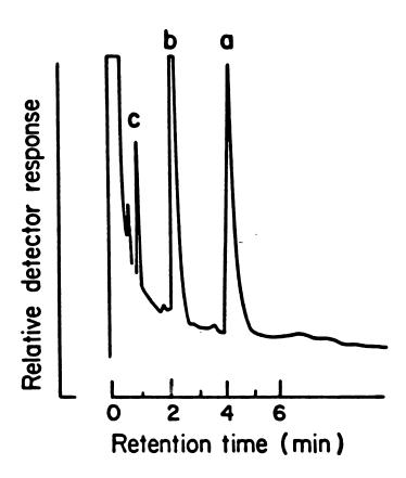
Gas-liquid chromatographic analysis of the extract from an incubation of phenylacetylene with microsomes from phenobarbital-induced rats. Methyl phenylacetate (a), methyl benzoate (the internal standard) (b), and phenylacetylene (c) are identified by the corresponding letter in the chromatogram.
