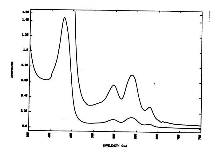
The electronic absorption spectrum of the DAP-PPIX adduct shows no shoulder on the soret band (430 nm). This is consistent with C or D ring alkylation.
