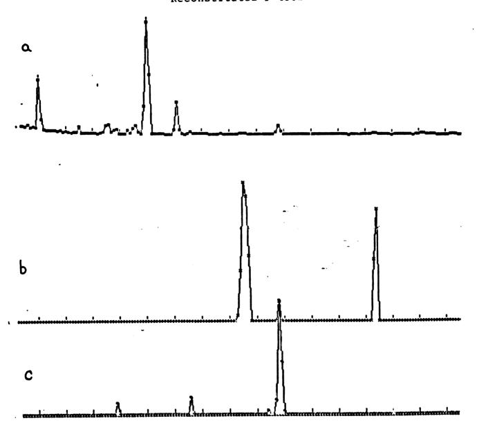
Gas chromatographic/mass spectrometric analysis of the methylated organic extract from an incubtation of (p-methylphenyl)acetylene with purified, reconstituted P-450b. A portion of the chromatogram is plotted showing (a) the total ions detected, (b) the total ions detected at m/e = 132 (the hydroxy methyl product) multiplied by 1024 and (c) the total ions detected at m/e = 164 (methyl p-methylphenylacetate) multiplied by 128.
