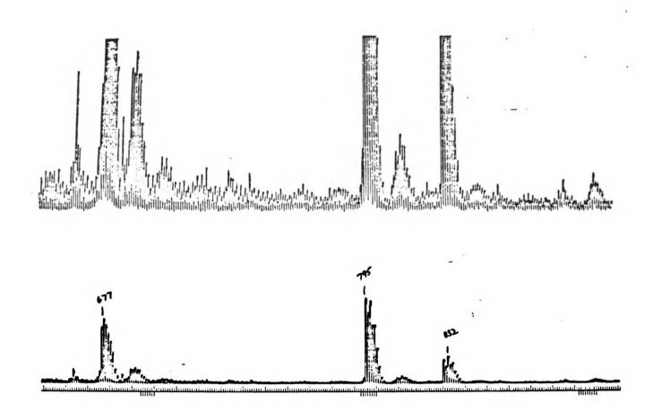
The zinc complex of the DAP-TPP adduct was prepared by treatment of the free base adduct with  $\text{Zn(OAc)}_2$  in methanol. The acetate counterion was exchanged for chloride, and the mass spectrum was recorded in tetraglyme. The molecular ion expected for the structure shown in Figure 5.21 is m/e 795, and the isotope pattern is that expected for a zinc complex.
