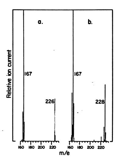
Mass spectra of methyl biphenylacetate obtained from incubations of biphenylacetylene with microsomes from phenobarbital-induced rats under (a) a normal atmosphere and (b) and atmosphere of  $^{18}\mathrm{O}_2$ . The lower mass regions are not shown.
