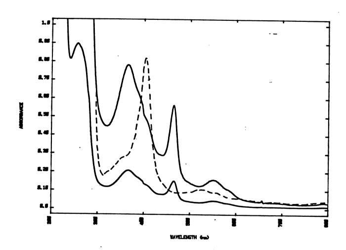
Electronic Absorption Spectra of Cytochrome  $b_5$  (----) and Manganese-Substituted Cytochrome  $b_5$  (----). The Manganese- $b_5$  shows the split Soret band typical of Manganese PPIX.
