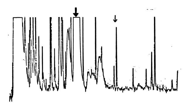
A 1:1 mixture of styrene and phenylacetylene was incubated with reconstituted P-450b to determine the relative rates of oxidation. The mixture was extracted as described in the text and the extracts were recombined and analysed. Styrene oxide is identified by the heavy arrow, and methyl phenylacetate by the light arrow.
