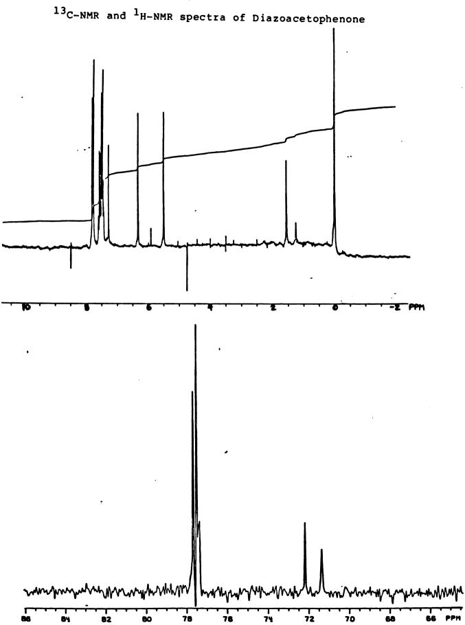
The  $^{13}$ C-NMR spectrum of DAP shows the carbon split by 204Hz. The  $^{1}$ H-NMR spectrum more accurately gave 198 Hz. The solvent is deuterochloroform which resonates at 77.5 in the  $^{13}$ C-NMR spectrum and 7.25 ppm in the  $^{1}$ H-NMR spectrum.
