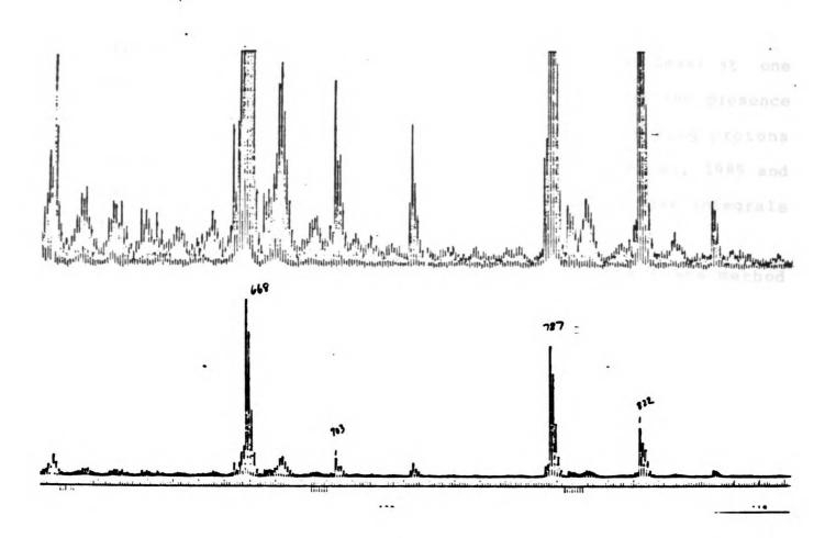
The LSIMS mass spectrum of the TPP-DAP complex in sulfolane shows the molecular ion at m/e 787 expected for the structure shown in Figure 5.16 as well as that for a chloride addition product at m/e 822 and fragments corresponding to TPP chloride (m/e 703) and TPP itself (m/e 668).
