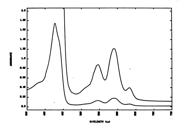
The electronic absorption spectrum of the EDA-PPIX adduct shows a soret band at 430 nm with the long wavelength shoulder indicative of A or B ring alkylation.
