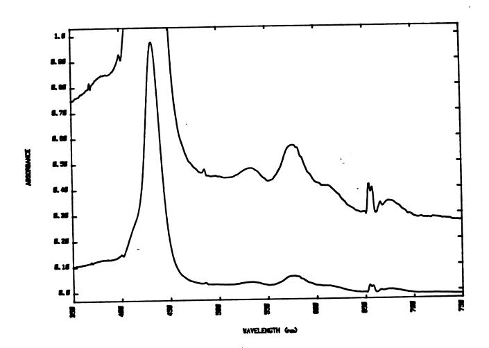
The TPP-DAP complex was demetallated over night with 5%  $\rm H_2SO_4/methanol$ . The electronic absorption spectrum has the expected soret maximum at 420 nm.
