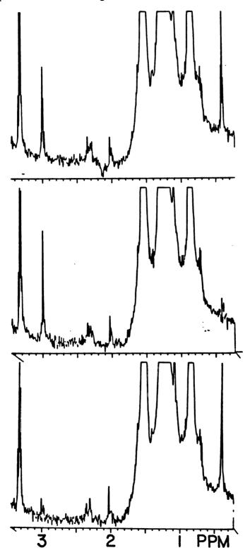
The ethoxy group protons in the EDA-PPIX adduct were identified by decoupling. (a) The undecoupled spectrum shows the methyl protons at 0.4 ppm coupled to the methylene at 3.0 ppm. (b) Irradiation of the methyl protons (indicated by the arrow) causes the methylene protons to become a singlet. (c) Irradiation of the methylene protons (indicated by 30 the arrow) causes the methyl group to become a singlet.
