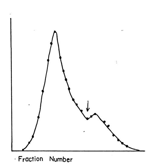
The amount of P-450 in each fraction was determined by monitoring the absorbance of the Soret (420 nm). The large peak is P-450b and the trailing peak P-450e.
