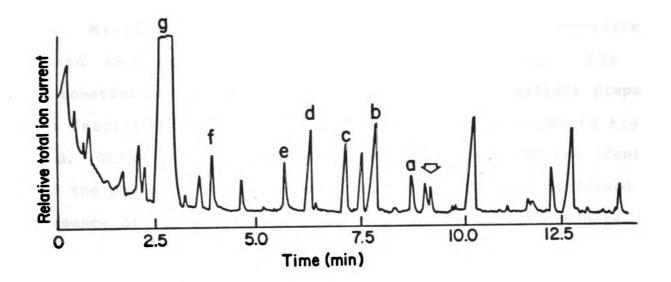
Analysis by GC/MS of the methylated organic fraction from the Fenton oxidation of phenylacetylene. The total mass spectrometric ion current is plotted. Methyl phenylacetate is indicated by the arrow. Other tentatively identified (retention time, mass spectrum) peaks are (a) 1-phenyl-1,2-ethanediol, (b) phenylacetone, (c) methyl benzoate, (d) acetophenone, (e) phenylacetaldehyde, (f) benzaldehyde, and (g) phenylacetylene.
