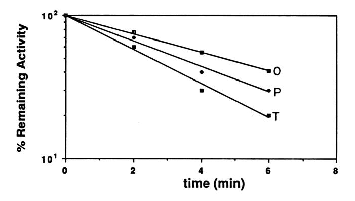
Inactivation of reconstituted P-450b caused by p-methyl (P), omethyl (O), and 2,4,6-trimethyl (T) phenylacetylenes.
