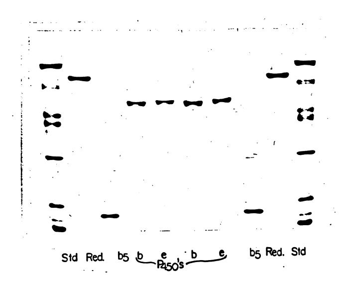
Purified P-450, Reductase and  $b_5$  were analysed by SDS Gel Electrophoresis. The lanes are labelled. Molecular weight standards (94, 67, 43, 30, 20, 14 kD) are in lanes 1 and 10.
