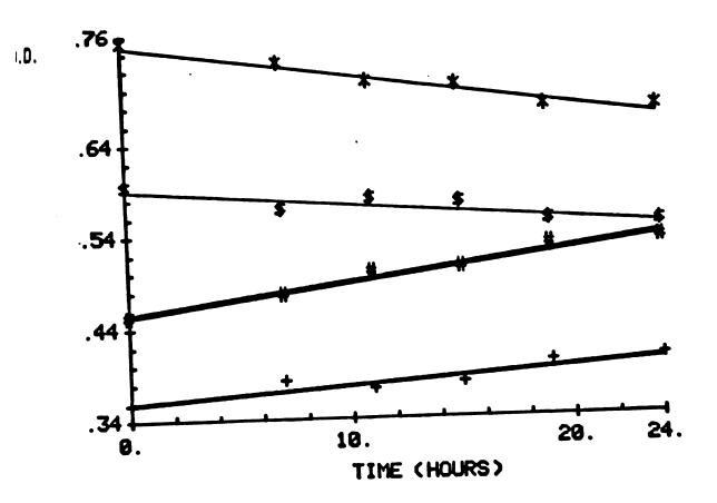
Analysis by electronic absorption spectroscopy of reactions of biphenylacetylene (\*,  $\ddagger$ ) or [1<sup>2</sup>H]biphenylacetylene (\$,  $\pm$ ) with metachloroperbenzoic acid in benzene solution containing 1% methanol (room temperature). The absorbance at 273 nm was monitored to determine loss of biphenylacetylene, and the absorbance at 255 nm was monitored to determine the production of methyl biphenylacetate.
