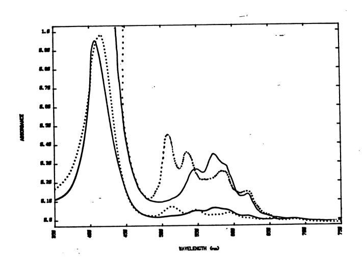
Approximately 10 ug of the PPIX-DAP adduct was dissolved in dichloromethane (----). Sulfolane was added neat until the spectrum indicated complete formation of the cation had occurred (\_\_\_\_\_). The amount of sulfolane required was 30 µl.
