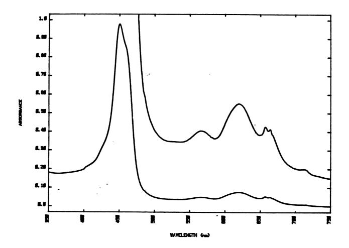
Diazoacetophenone was reacted with TPPFe(II) under anaerobic, reducing conditions. A stable product with a Soret band at 455 nm was immediately formed.
