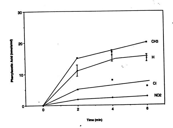
Concentrations of the substituted phenylacetic acid metabolites as a function of time of incubation of substituted phenylacetylenes with reconstituted cytochrome P-450b. The substituent on the phenylacetic acid is indicated. The experimental conditions are given in Chapter 2. The standard deviations for phenylacetic acid production are indicated by bars. The standard deviations for the other measurements are similar but are not shown for the sake of clarity.
