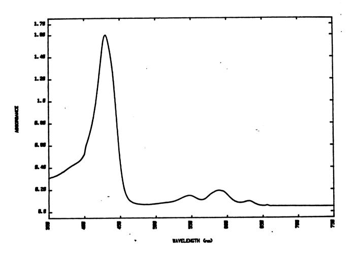
Purified P-450b was incubated with diazoacetophenone and then reduced with excess  $Na_2S_2O_4$  to form the 445 nm complex. The mixture was mixed with 5%  $H_2SO_4$ /methanol and analysed for N-alkyl porphyrin formation. The electronic absorption spectrum of the DAP-PPIX adduct thus isolated is identical to that shown in figure 5.9.
