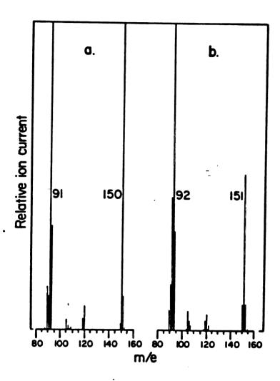
Mass spectra of methylphenylacetate obtained from microsomal incubations of (a) phenylacetylene and (b) [1-2H] phenylacetylene. The lower mass regions are not shown.
