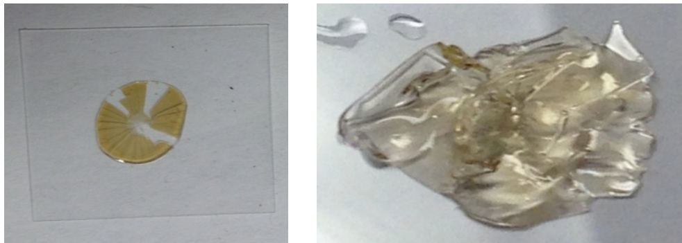
Figure 3.8 Left: dried polymer film. Right: when the film is dipped into water, it swells to form a gel.
