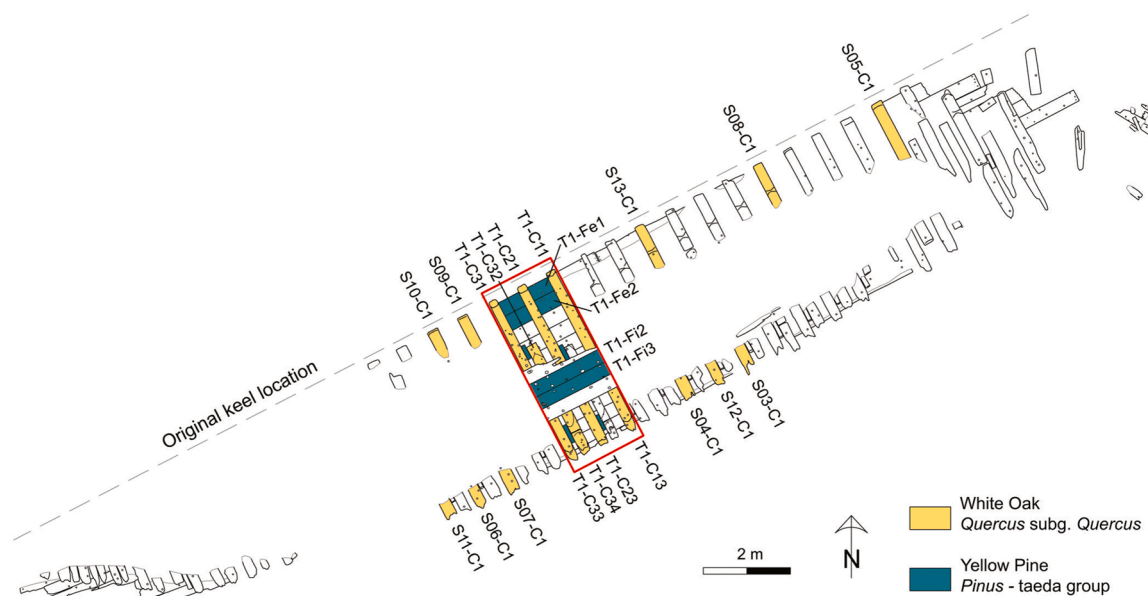
Fig. 3. Plan of BG2 structure with the location of the sampled timbers. Trench T1 is located in the central part of the structure (red rectangle). To facilitate the reading of the figure, the legends for the spacer blocks have been omitted (drawing C. Murray).
