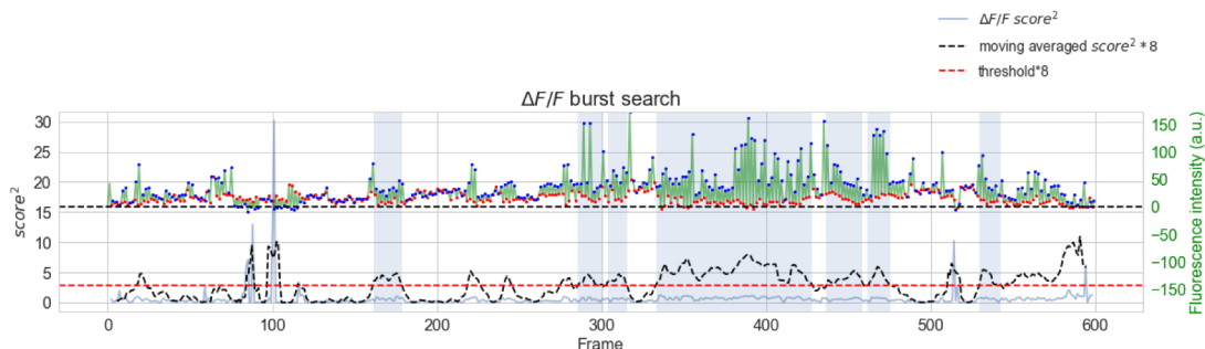
Fig. S5-6: An example result for \Delta F/F burst search applied to the intensity trace from a type-II ZnSe/CdS NR. The blue line is the \Delta F/F score^2 . The black dashed line is the 8\times moving averaged score^2 with a window of 8 frames. The red dashed line is the 8\times threshold above which the “start” of a burst will be identified. For this NR, 7 bursts above the threshold (and above the time threshold of 8 frames) were detected and marked by the blue shaded areas. The green line is the intensity ( F ) trace with the scale indicated on the right, and the blue and the red dots mark the F 's at V_{on} and V_{off} frames, respectively.
