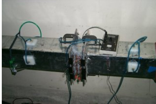
Figure 8. Measurement of the coil pressure drop
