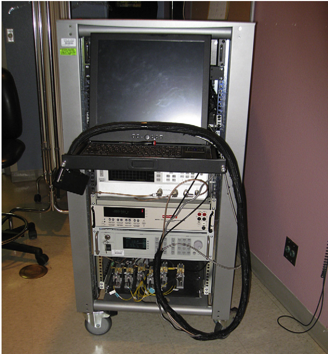
Figure 1. Current Diffuse Optical Spectroscopic Imaging (DOSI) instrument. The DOSI instrument measures tissue complete absorption and scattering spectra from 650 to 1000 nm through the use of a handheld probe (seen on top of system). Spectroscopic images are generated by translating the handheld probe along a rectilinear grid on the surface of the breast.
