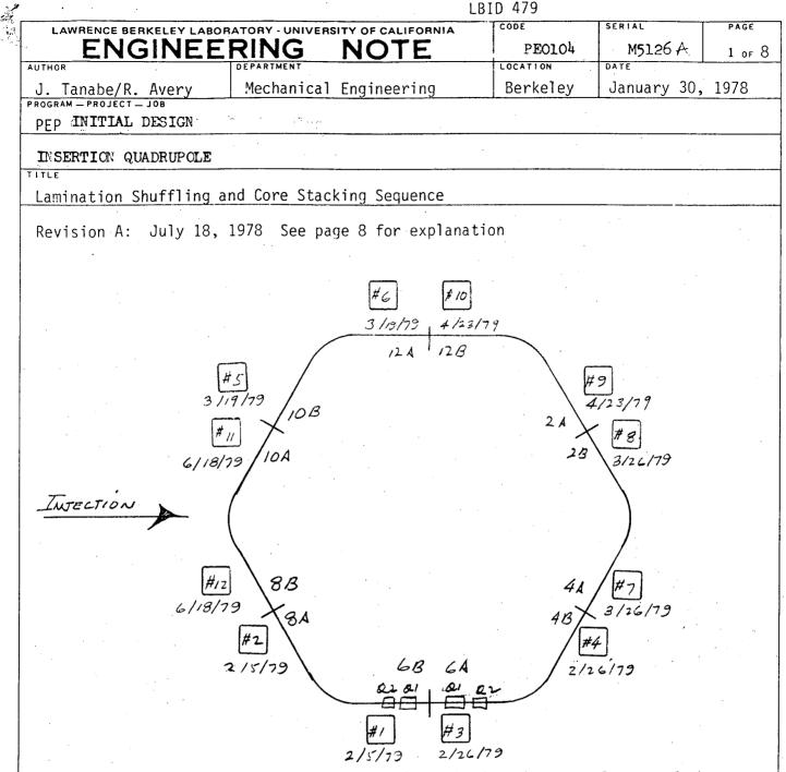
The above is a schematic of the PEP ring, showing the nomenclature of the interaction regions, showing the position of the interaction quadrupoles in each region.
