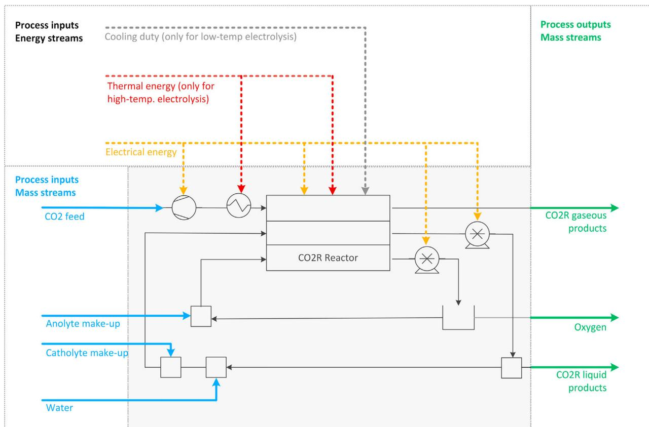
**Figure 3. Overview of the CO<sub>2</sub>R reactor with possible related unit operations**
