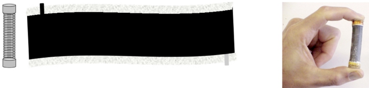
Figure 1.21: Spring roll DEA. Rolls are fabricated by compressing a spring between two end caps and rolling a DE/electrode/DE/electrode layered strip around it. Increasing the number of layers wrapped around the spring core increases the output force. [249] Proc SPIE 2003, reprinted with permission.
