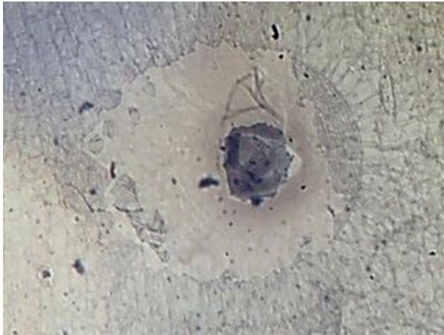
Figure 1.20: Cleared area on a CNT electrode. Localized dielectric breakdown results in an electrical short through the film. Corona discharging burns away the CNTs in the area surrounding the short, isolating it from the rest of the electrode and allowing the device to continue operating.
