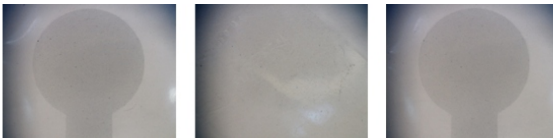
Figure 5.1: SWNT electrodes on S-IPN film. Left to right: as deposited, post-cure electrode after one adhesion test, pre-cure electrode after multiple adhesion tests.
