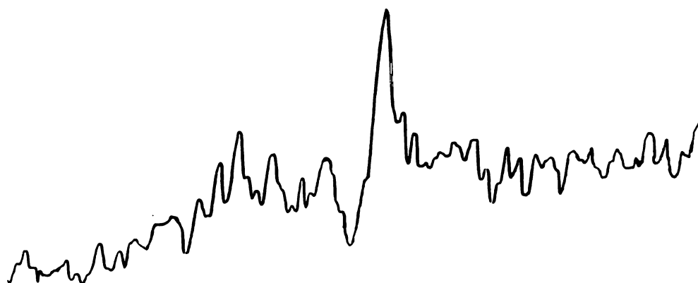
Figure 4.3.7. EPR spectrum of 8F-HRP upon addition of hydrogen peroxide.
