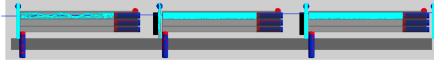
Figure 10.15: Rendering of a beam-based mCP traveling through a GEANT4 model of the demonstrator, hitting all four slabs and three bars in a straight line. Light blue lines are generated optical photons.
