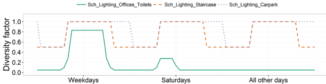
Figure 5: Lighting power demand schedules in benchmark model for three different week day types.
