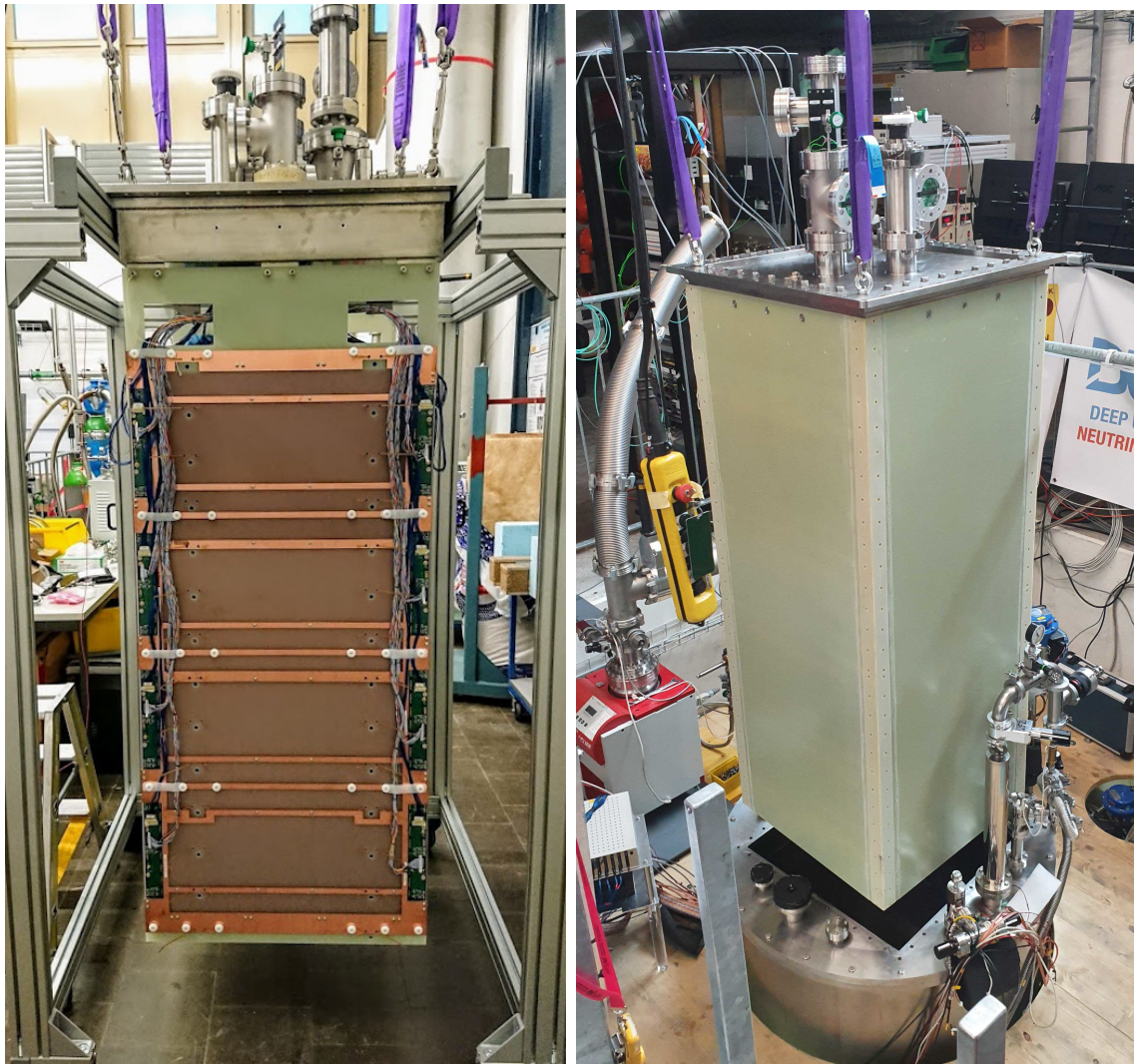
Figure 4.3: (Left) Fully assembled Module 0. (Right) Module 0 being lowered into the cryostat.
