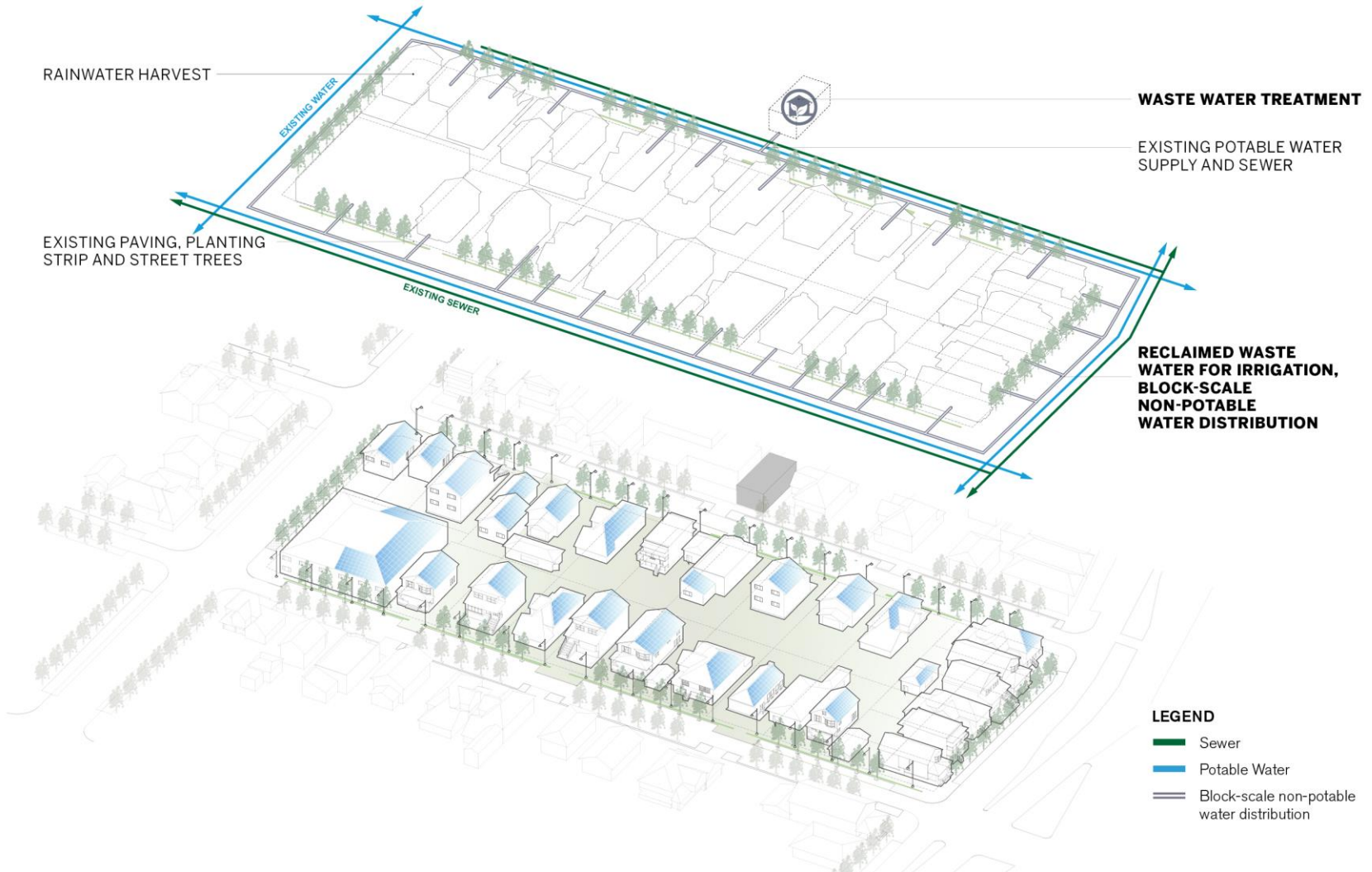
Bolt-on C: Sewer Mining—Reclamation for Irrigation for Non-Potable Water at Neighborhood Scale. Credit: Skidmore, Owings & Merrill, LLP
