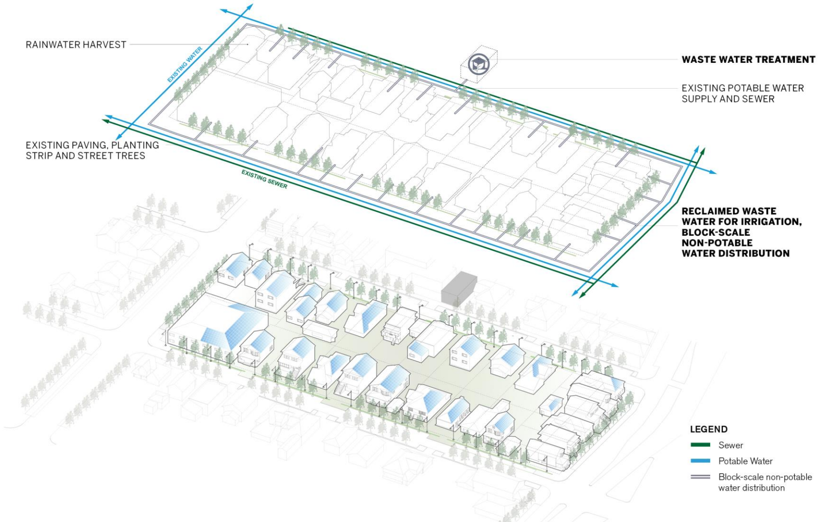
Bolt-on C: Sewer Mining—Reclamation for Irrigation for Non-Potable water at the Neighborhood Scale. Source: Skidmore, Owings & Merrill, LLP
