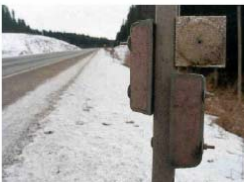
(Figure 21). Wildlife warning reflectors subjected to winter roadside conditions
