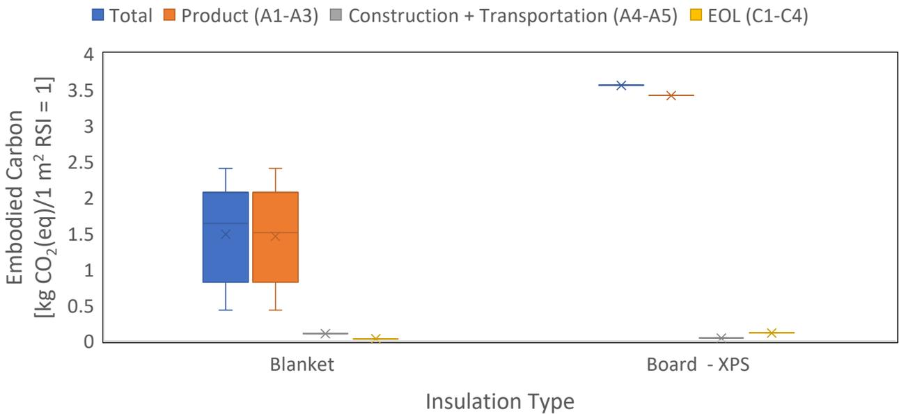
Figure 20. Range of embodied GHG values, in units of kg CO<sub>2</sub> (eq) per functional unit (1 m<sup>2</sup> of insulation at an RSI =1), by floor insulation type and life-cycle stage. All EPDs for this product are sourced in the United States/North America. The embodied carbon footprint of foamed-in-place insulation is approximately 5 times greater than board insulation and is approximately 5 times and almost 25 times greater than blown insulation in wall and ceiling applications.
