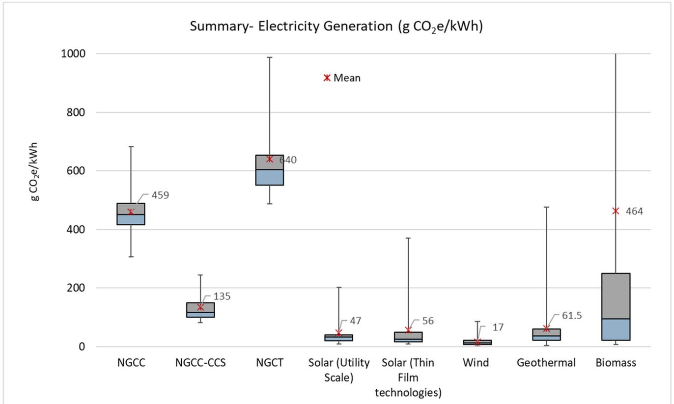
Figure 16. Variability in GHG emission factors calculated for targeted electricity generation technologies.
