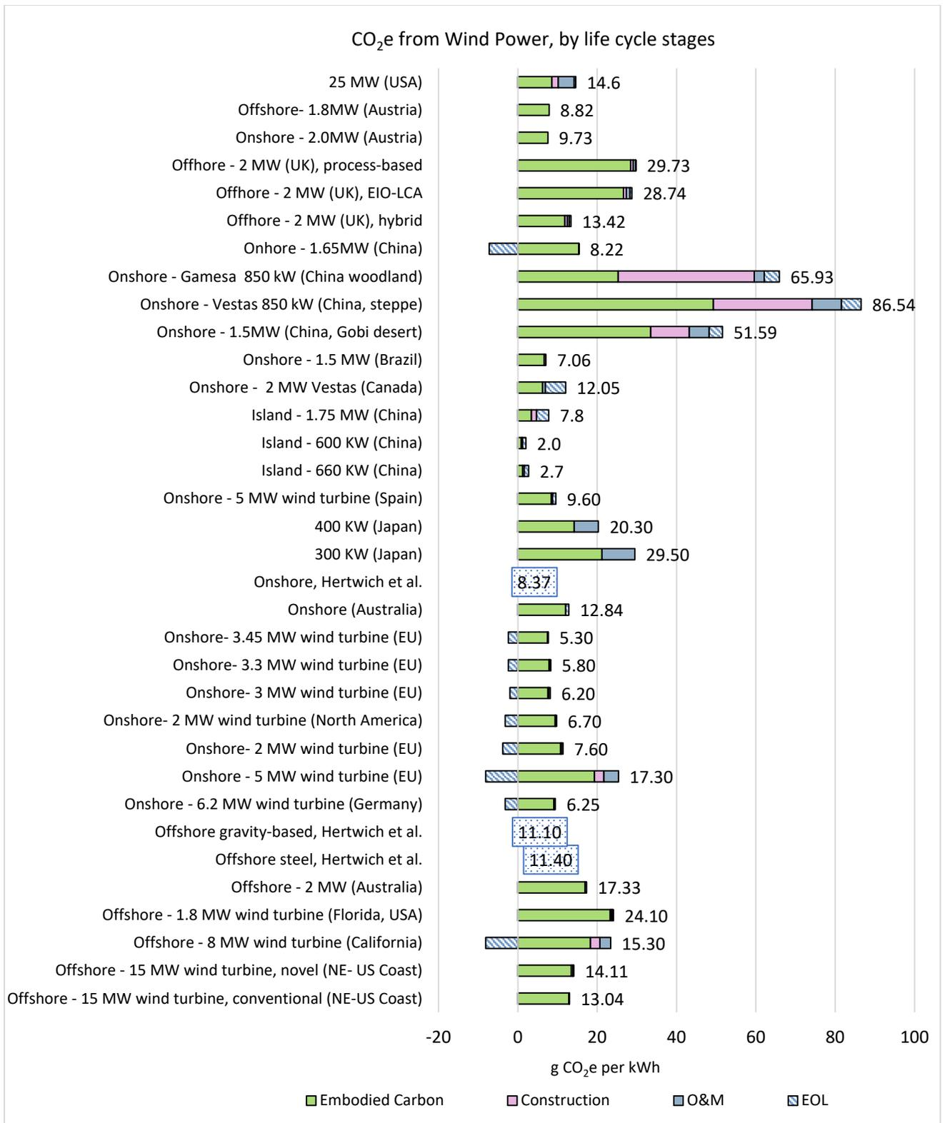
Figure 10. Life-cycle GHG emissions of various wind power systems based on literature and manufacturer EPDs<sup>25,40-70</sup>.
