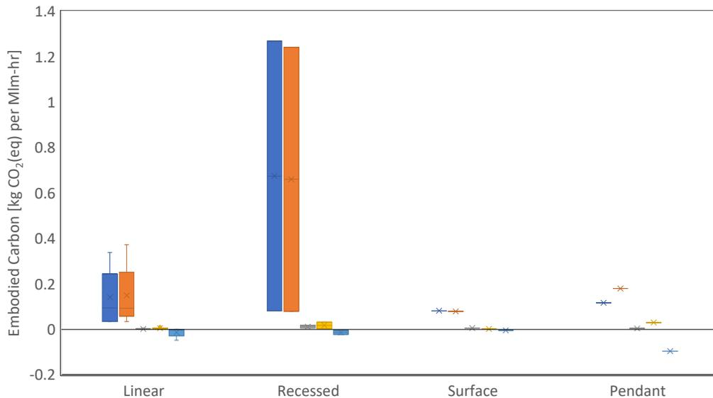
Figure 30. Embodied GHG values, in units of kg CO<sub>2</sub> (eq) mega lumen-hour, for various indoor lamp types.
