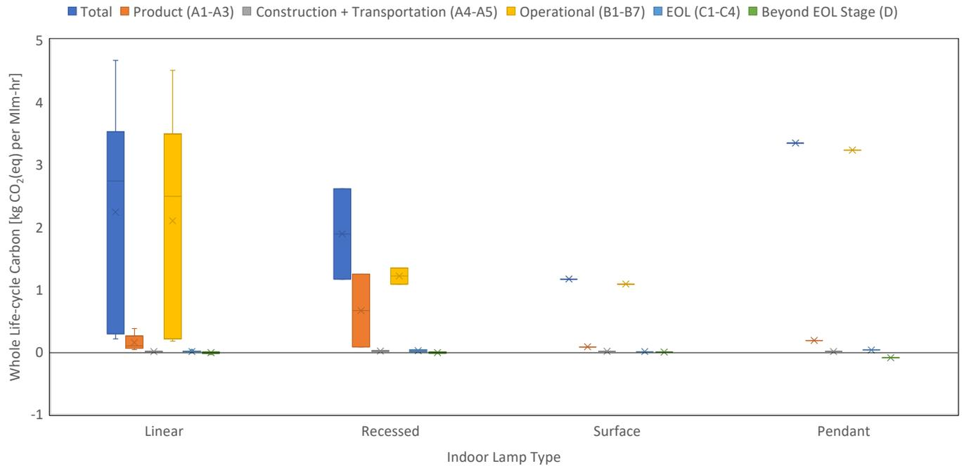
Figure 29. Life-cycle GHG emissions, in units of kg CO<sub>2</sub> (eq) mega lumen-hour, for various indoor lamp types.
