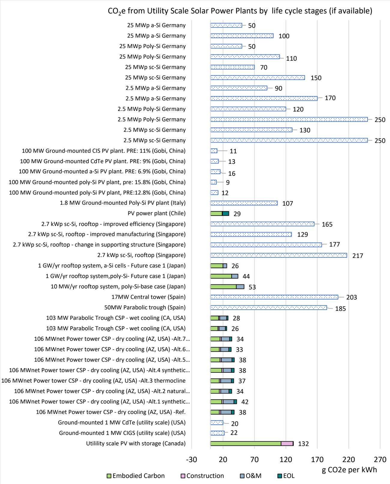
Figure 5. Life cycle GHG emissions of various utility-scale and rooftop solar power systems based on literature and manufacturer EPDs<sup>12,16-38</sup>.
