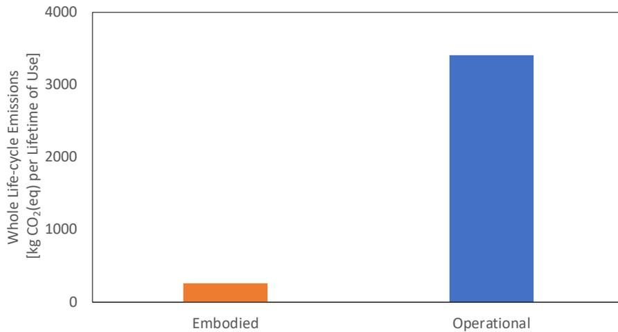
Figure 34. Embodied and operational GHG emissions, in units of kg CO<sub>2</sub>(eq) per lifetime of use, for a residential dishwasher.
