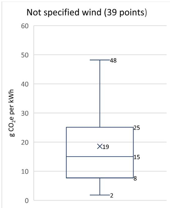
Figure 9. The box the 25th to 75th percentile, and the whisker the 2.5th to 97.5th percentile. Underlying data for the results from 99 articles and reports from the literature review<sup>25,40-70</sup>.
