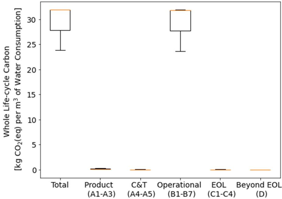
Figure 24. Life-cycle GHG emissions, in units of kg CO<sub>2</sub>(eq) per m<sup>3</sup> of water consumption, for commercial and residential showerheads.
