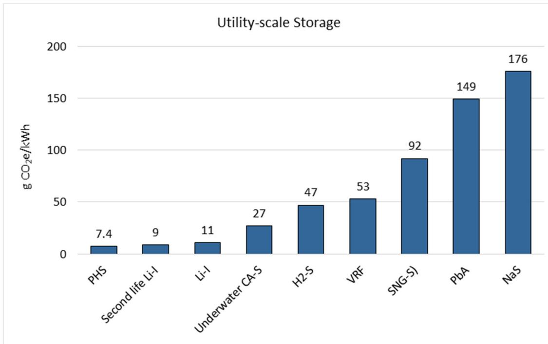
Figure 14. the GHG emission factors estimated for utility-scale storage systems<sup>77</sup>. Note: Li-I-B: lithium-ion battery, NaS: Sodium-sulfur battery, PbA: Lead-acid battery, SL-Li-I: Second-life battery, SNG-S: power-to-gas synthetic natural gas storage, VRF: Vanadium redox flow battery
