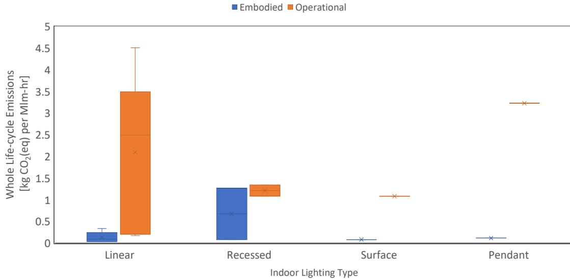
Figure 33. Breakdown between embodied and operational GHG emissions, units of kg CO<sub>2</sub> (eq) mega lumen-hour, for various indoor lighting types.
