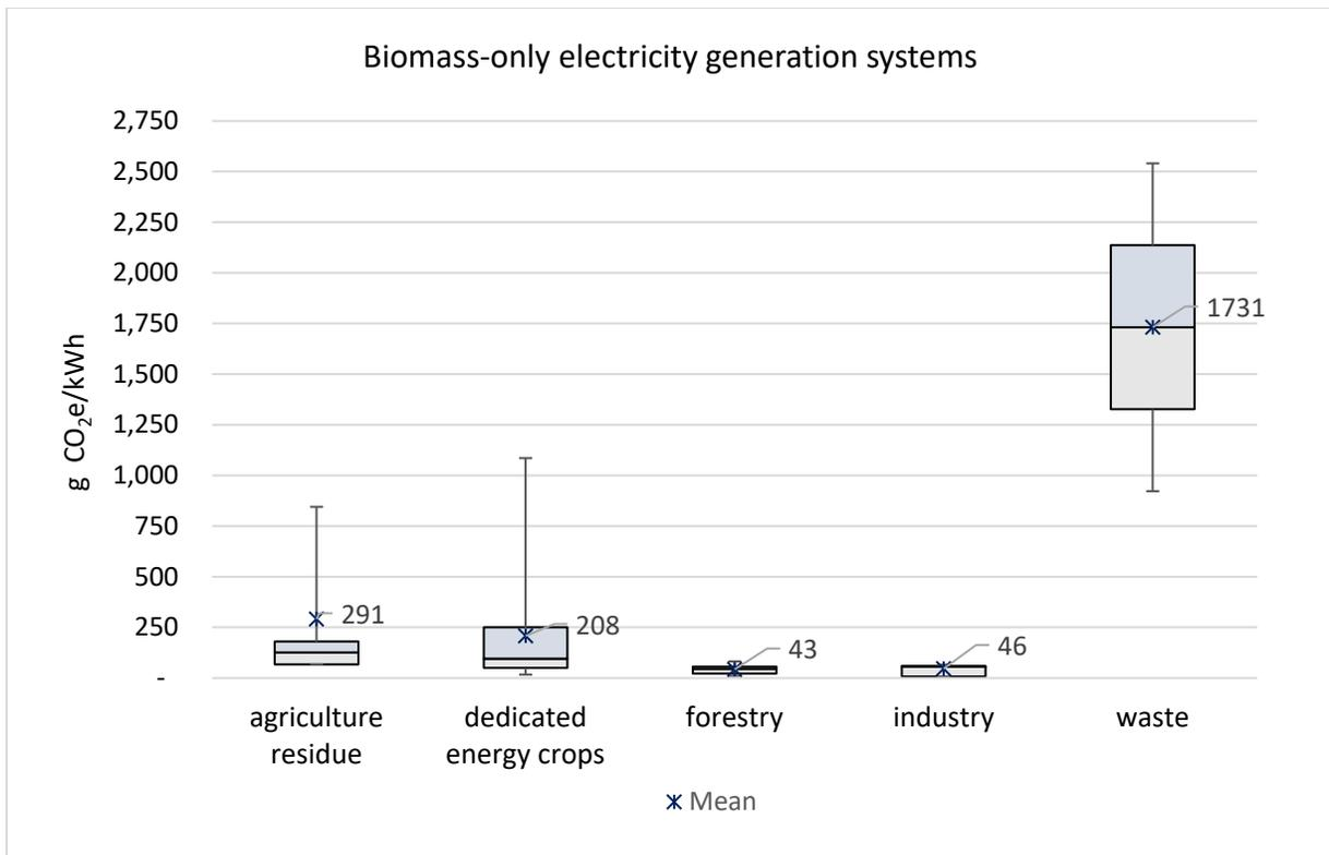
Figure 13. GHG emission (gCO<sub>2</sub>e/kWh) statistics from biomass-only electricity generation systems<sup>30</sup>.
