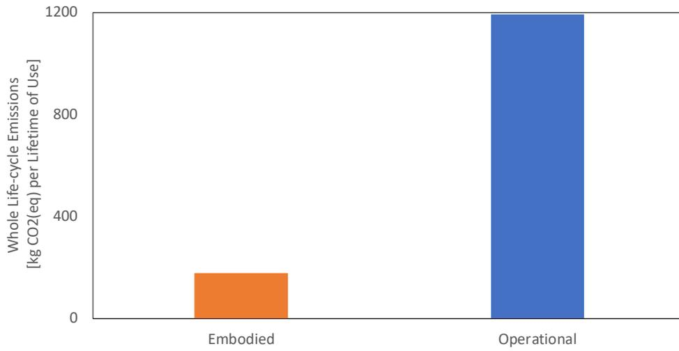
*Figure 35. Embodied and operational GHG emissions, in units of kg CO<sub>2</sub> (eq) per lifetime of use, for a residential electric clothes dryer.*
