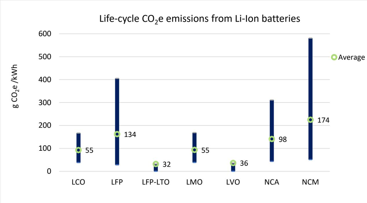
Figure 15. Life cycle GHG emissions of lithium-ion batteries
