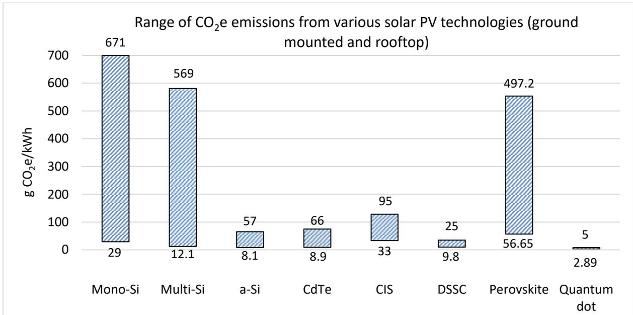
Figure 7. Life cycle GHG emissions of solar photovoltaic electricity generation technologies (Source: NREL website: <https://www.nrel.gov/analysis/life-cycle-assessment.html>)
