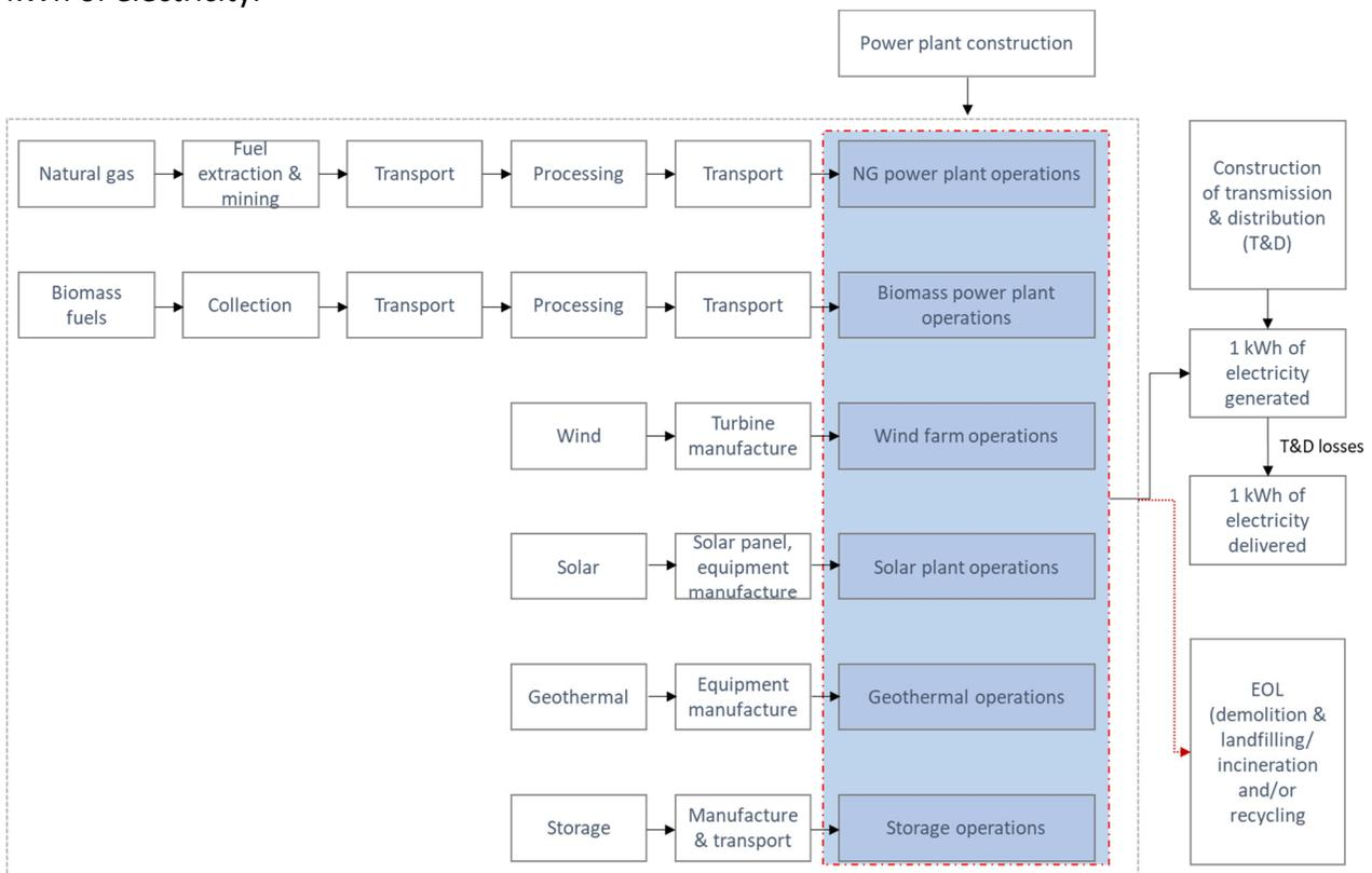
Figure 3. An illustrative scope of targeted electricity generation and storage types and cradle-to-grave life cycle stages represented in the analysis.
