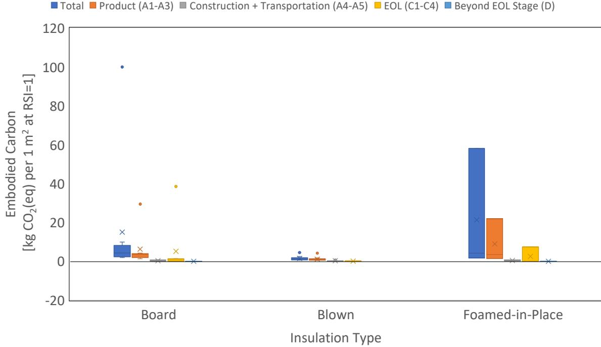
Figure 21. Range of embodied GHG values, in units of kg CO<sub>2</sub>(eq) per functional unit (1 m<sup>2</sup> of insulation at an RSI =1), by insulation type and life-cycle stage. Applies for commercial and residential wall and ceiling insulation. All EPDs for this product are sourced in the United States/North America.
