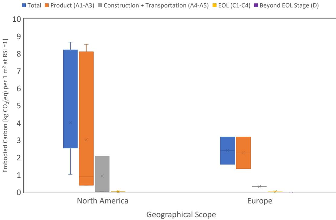
Figure 22. Range of embodied GHG values, in units of kg CO<sub>2</sub>(eq) per functional unit (1 m<sup>2</sup> of insulation at an RSI =1), for HVAC duct insulation by geographical scope and life-cycle stage.
