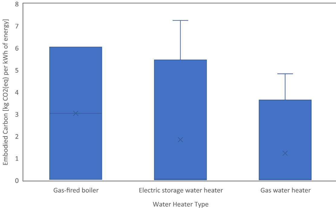
Figure 28. Embodied GHG values, in units of kg CO<sub>2</sub> (eq) per kWh of energy needed to heat water, for various water heater types.
