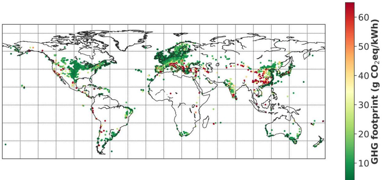
Figure 8. Greenhouse gas footprints of the individual wind farms in g CO<sub>2</sub>eq/kWh of the global wind farm fleet<sup>42</sup>.
