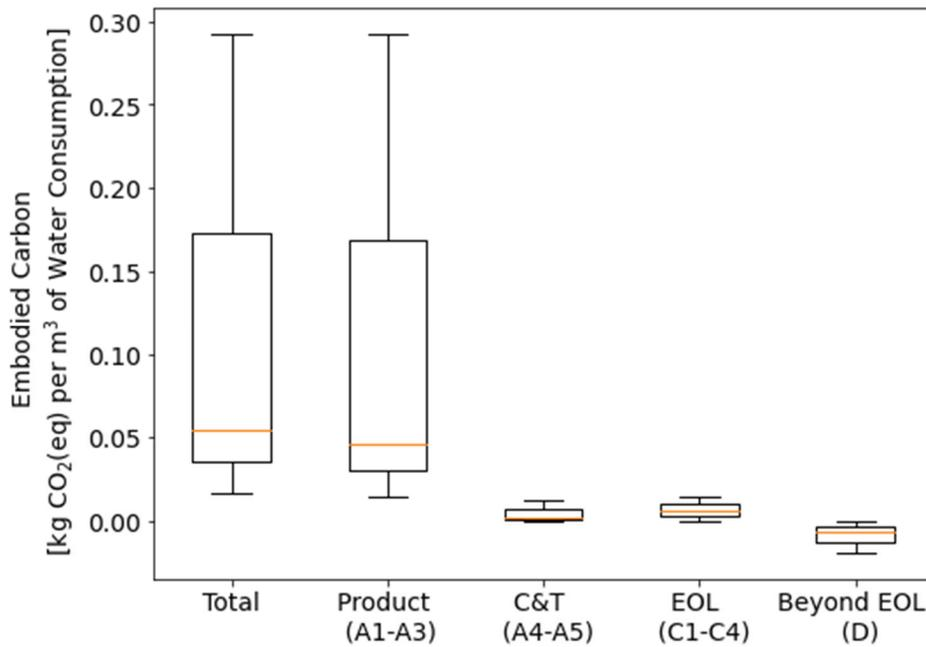
Figure 25. Embodied GHG values, in units of kg CO<sub>2</sub>(eq) per m<sup>3</sup> of water consumption, for commercial and residential showerheads.
