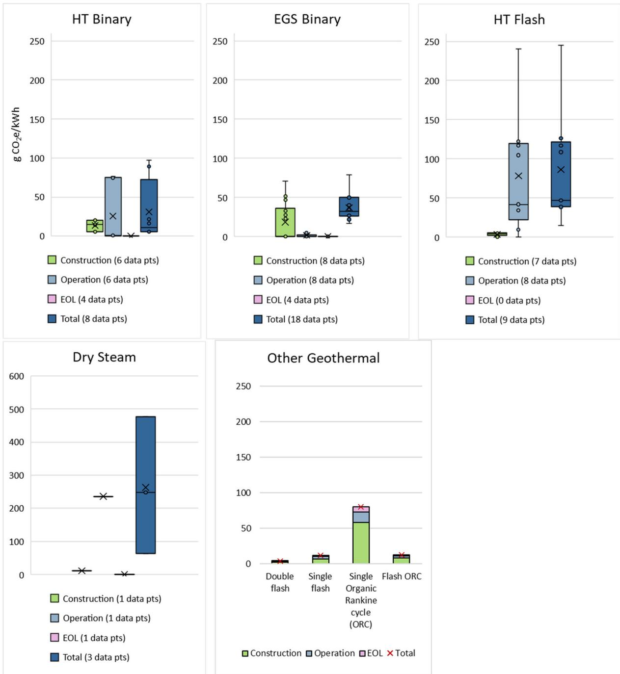
Figure 11. Lifecycle GHG emissions of geothermal power generation<sup>50,71-76</sup>.
