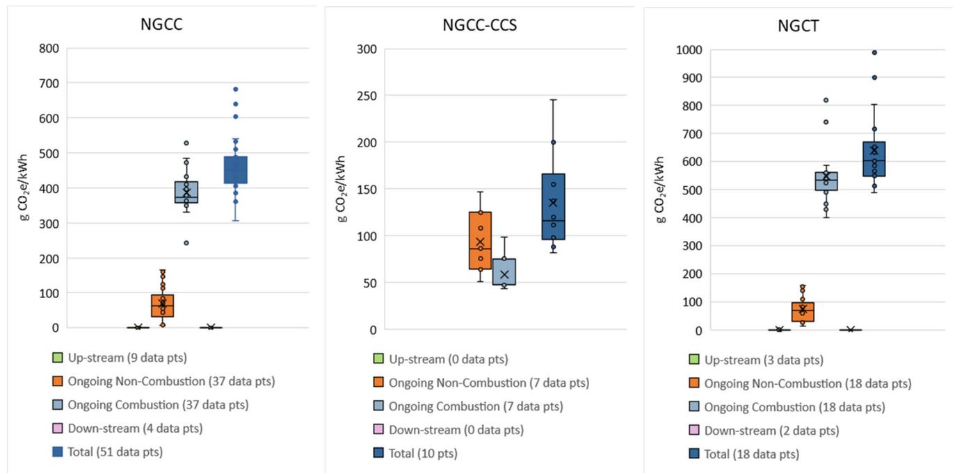
Figure 4. Cradle-to-grave life cycle GHG emissions from various natural gas power plants based on literature review adapted from O’Donoughue et al<sup>12</sup>. Note: NGCC - natural gas combined cycle; NGCC-CCS - natural gas combined cycle with carbon capture and storage; NGCT - natural gas combustion turbine.
