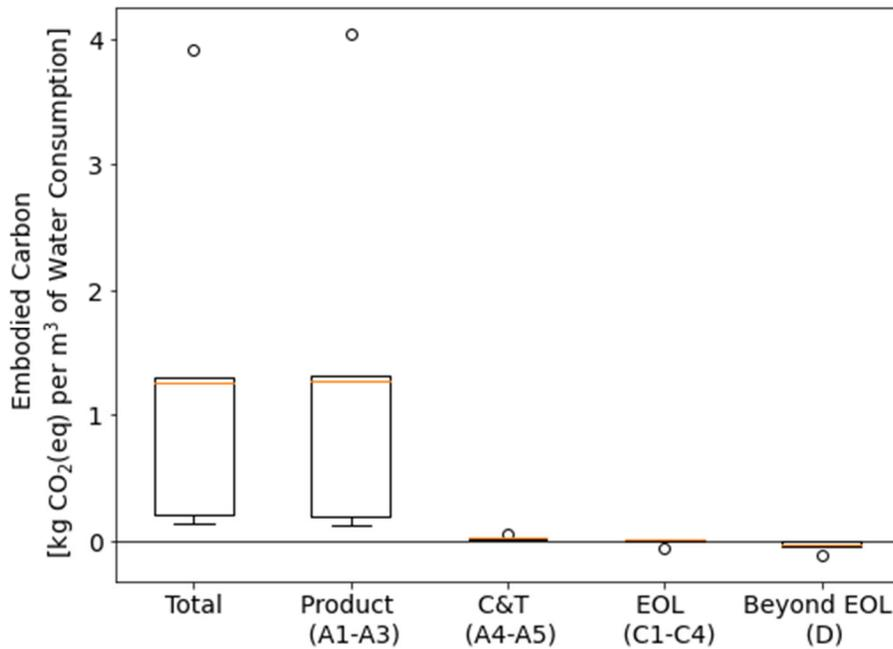
Figure 27. Embodied GHG values, in units of kg CO<sub>2</sub>(eq) per m<sup>3</sup> of water consumption, for commercial and residential faucet aerators.
