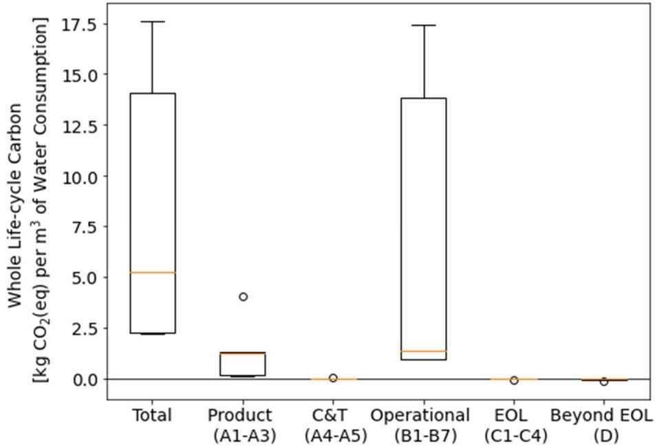
Figure 26. Life-cycle GHG emissions, in units of kg CO<sub>2</sub>(eq) per m<sup>3</sup> of water consumption, for commercial and residential faucet aerators.
