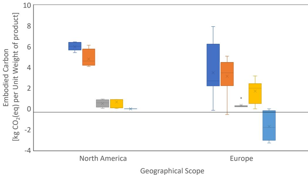
Figure 23. Range of embodied GHG values, in units of kg CO<sub>2</sub>(eq) per unit weight of product, for pipe insulation by geographical scope and life-cycle stage.
