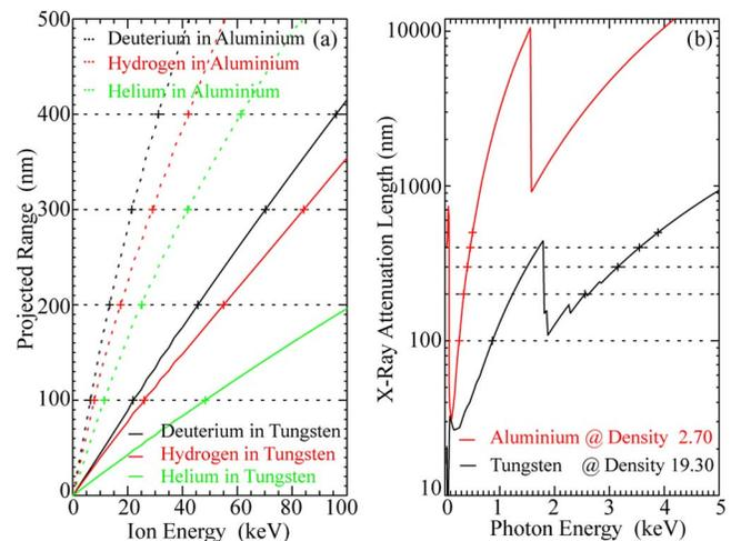
FIG. 1. Ion projected range from SRIM calculation (a) and X-ray transmission length (b) in tungsten (W) and aluminium (Al) foil.
