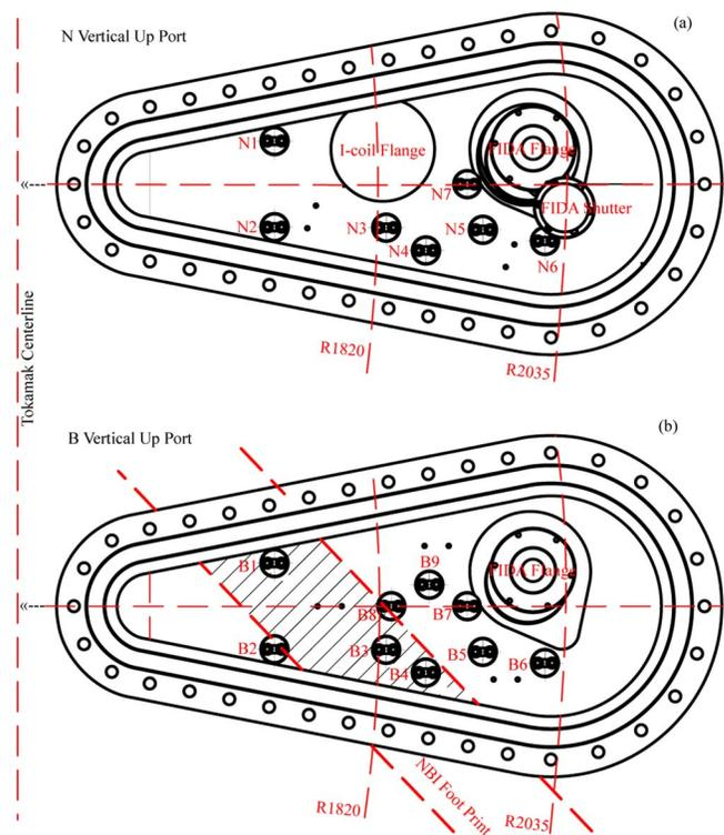
FIG. 3. Locations of individual vertical ssNPA detectors.
