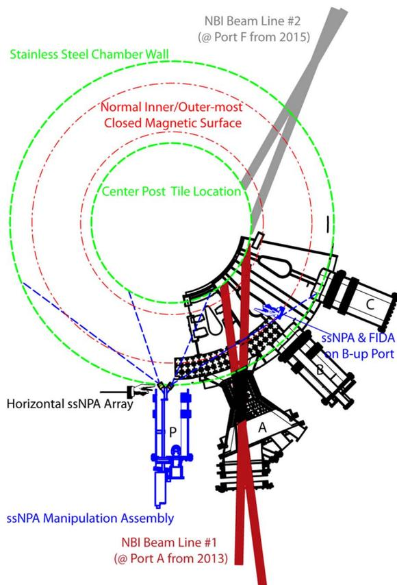
FIG. 2. NBI footprint locations and ssNPA field of view.
