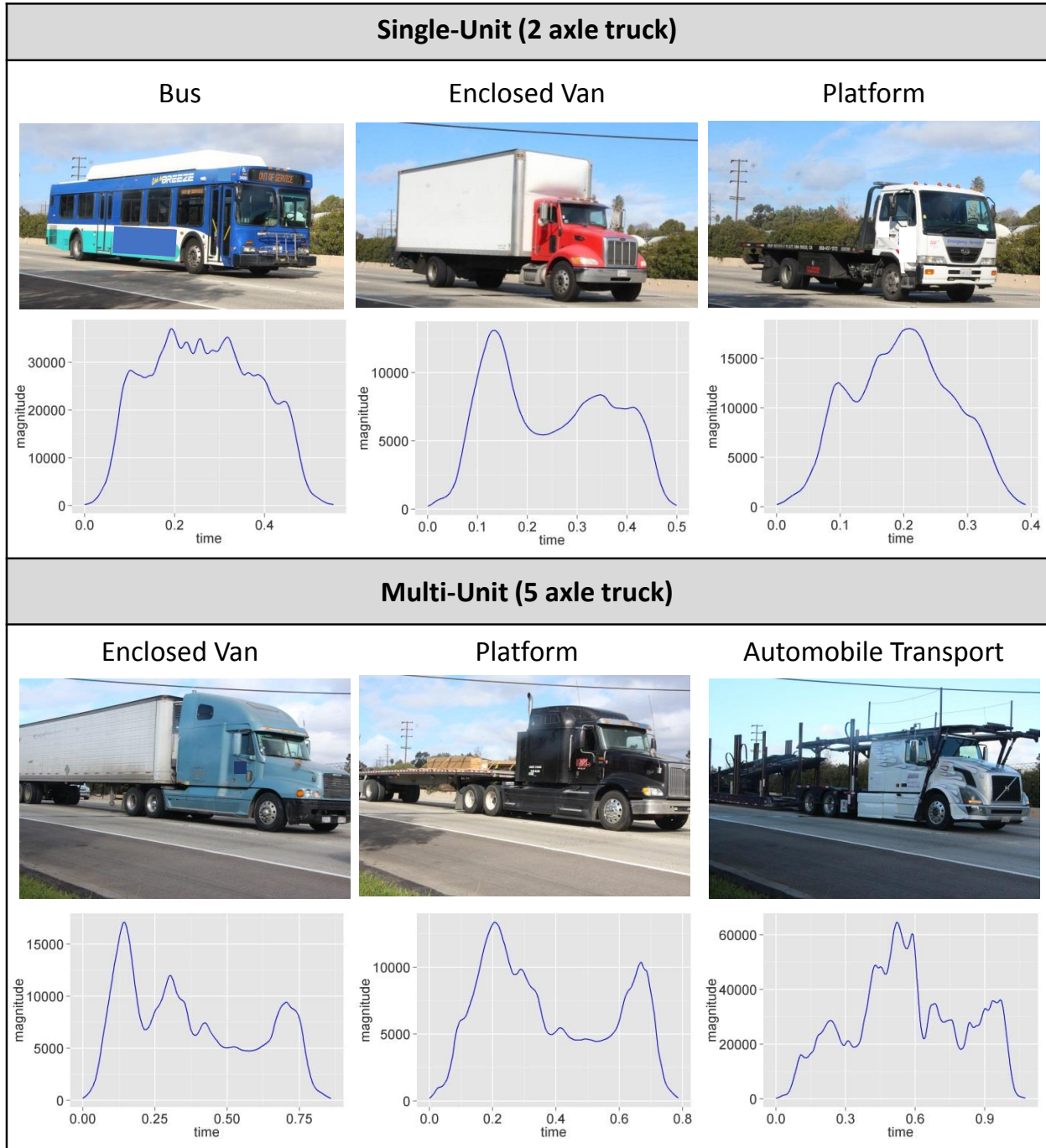
Figure 2.5 Signature from different truck body configuration
