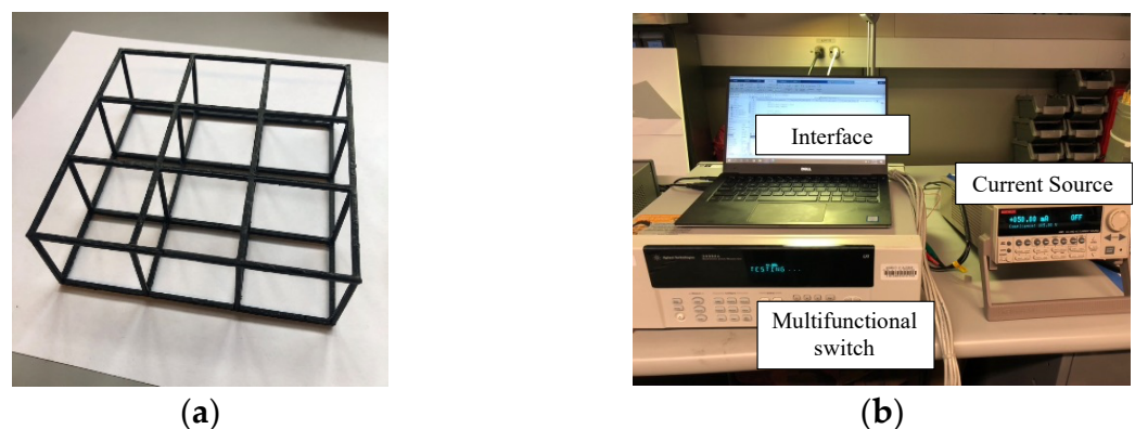
Figure 10. (a) A 3 \times 3 \times 1 lattice structure was spray-coated with a conductive, nanocomposite thin film. (b) ERT measurements were obtained using a customized data acquisition system.
