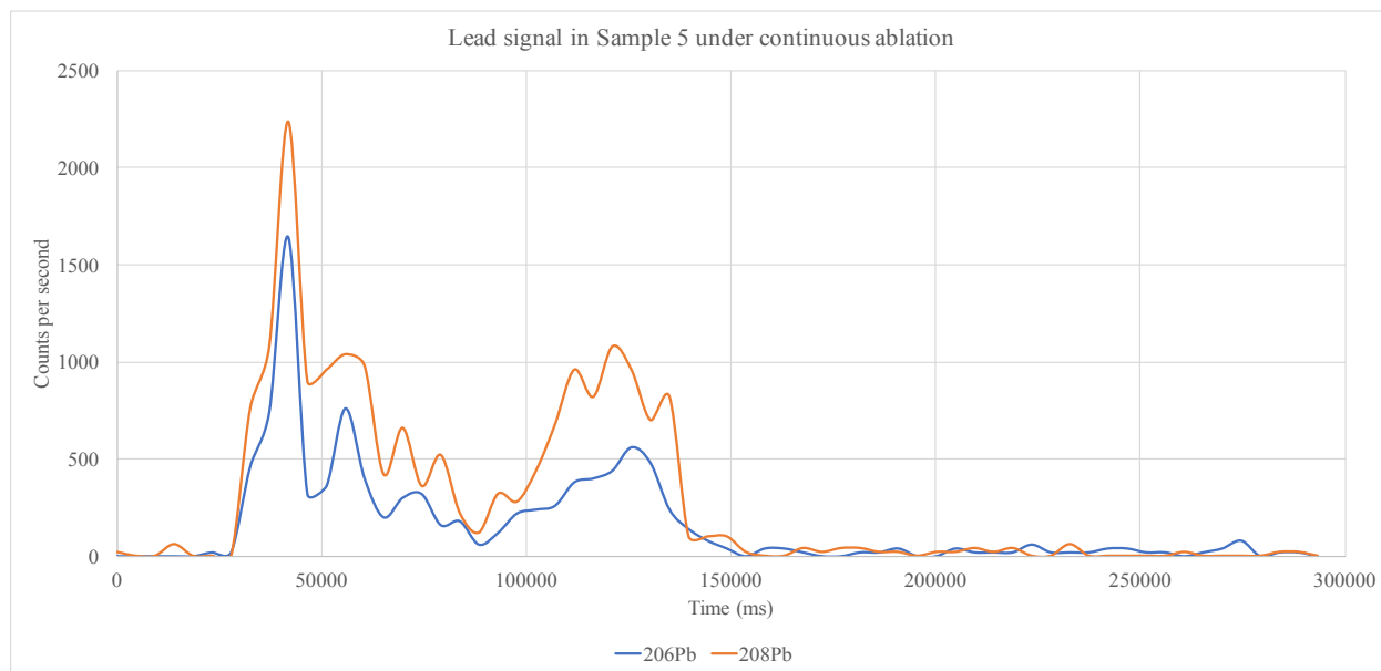
Figure 7.43: Lead signal in Sample 5 under continuous ablation.
