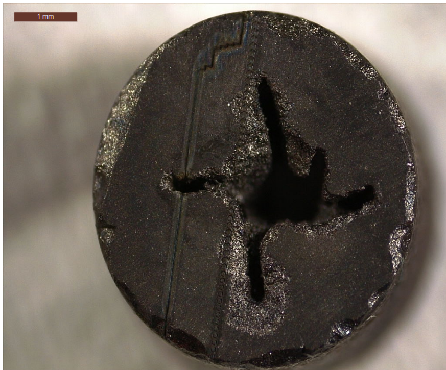
Figure 7.21: Optical image of ablation tracks across the end of Sample 5.
