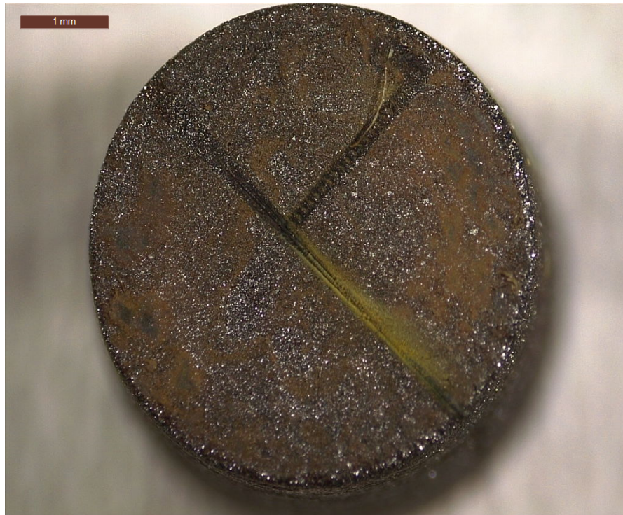
Figure 7.12: Optical image of Sample 2 showing an overview of the impact of surface height variation on laser ablation efficiency.
