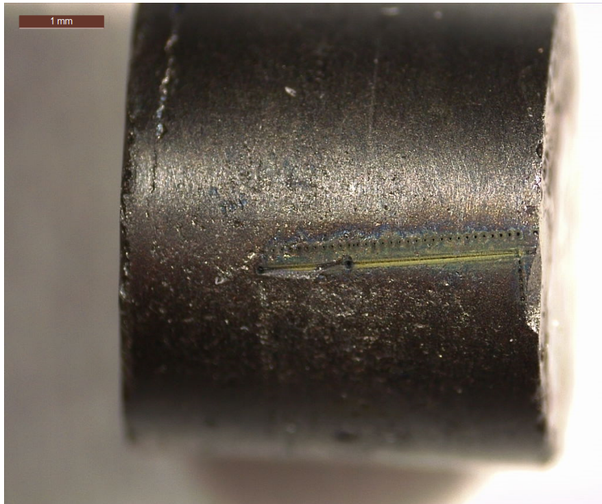
Figure 7.17: Optical image of a truncated ablation track along the axis of Sample 4.
