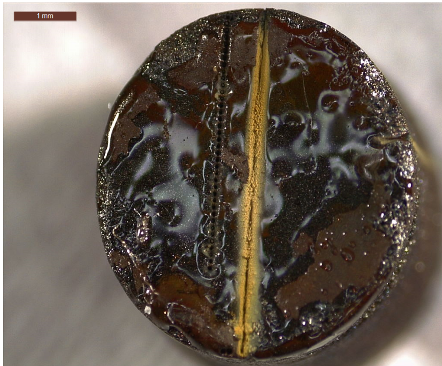
Figure 7.15: Optical image of stepped and continuous ablation tracks through variable surface texture across the end of Sample 3.
