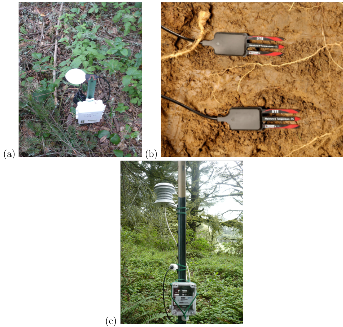
Figure A.2: a) Leaf wetness sensor (Decagon LWS); b) soil moisture sensor (Decagon 5TM time domain reflectometers); and c) weather station (HOBO H21-002 Micro Station).
