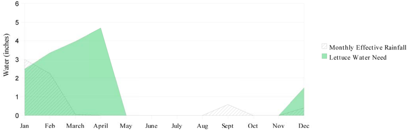
Effective Rainfall versus Water Need for Lettuce in Sacramento Example 1: Winter-planted Lettuce
