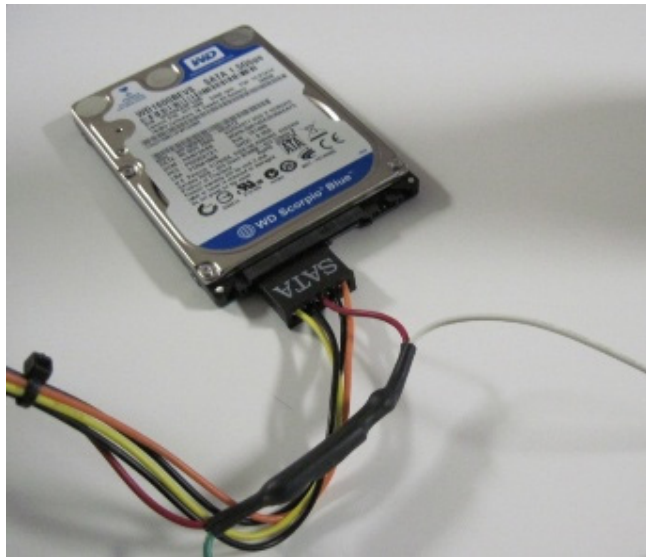
Figure 2.3. SATA hard drive with instrumented power supply cable containing a 0.1\Omega current sensing resistor.
