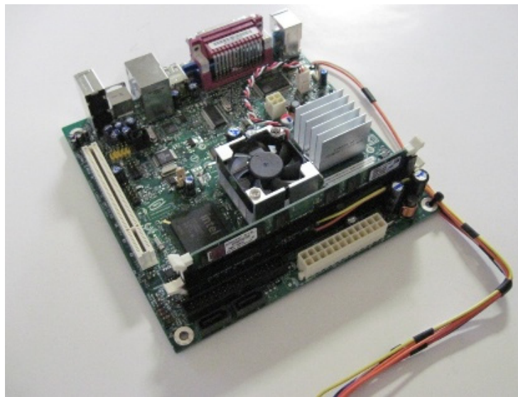
Figure 2.4. The Atom board with the memory module in the foreground. A riser card with a current sensing resistor attaches the memory module to the board.
