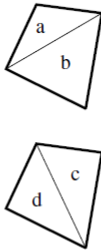
Figure 7-2 Sets of triangles in a quadrilateral element (Itasca Consulting Group 2011)
