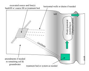
AEMP should also consider installing a high permeability backfill material to facilitate controlled drainage, possibly including amendments such as reducing agents and/or a
