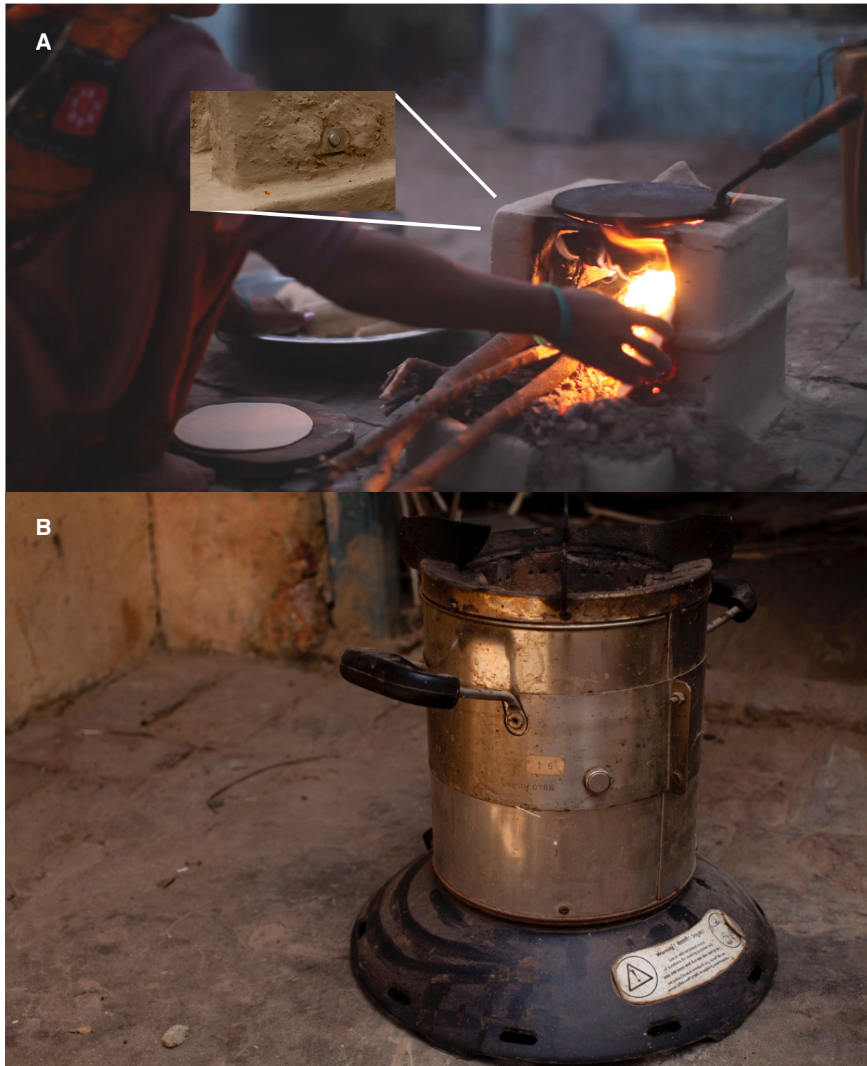
Figure 4.1 Traditional and intervention stoves and placement of stove use monitors A is a typical traditional wood and dung-fueled stove. The inset image shows the Stove Use Monitor and its holder. B is the Philips intervention stove. A metal sheet stamped with a unique identifier and machined with a hole was used to securely hold each stove use monitor.
