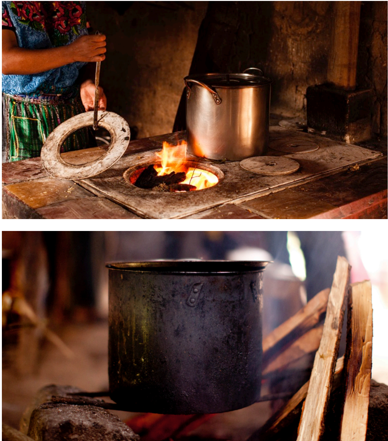
Figure 2.1 Typical intervention and traditional stoves in San Lorenzo, Guatemala The top panel depicts the Plancha intervention stove in San Lorenzo, Guatemala. Fuel is fed into an enclosed combustion chamber (not visible); smoke vents out through a chimney (near the rear of the stove). The lower panel depicts a typical open fire cookstove.
