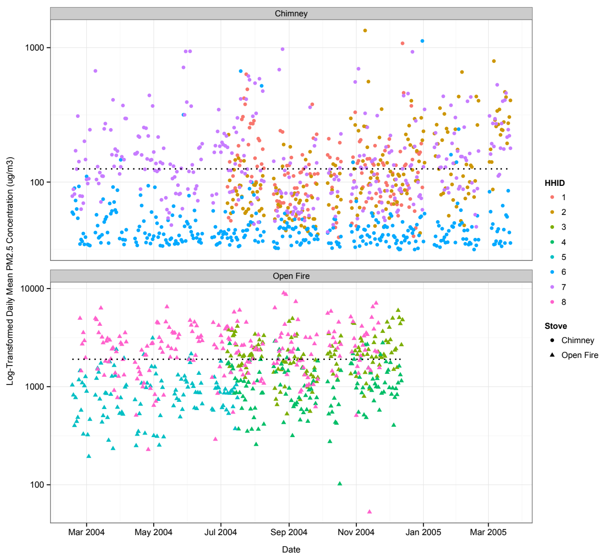
Figure 2.2 Daily mean PM 2.5 concentrations in \mu\text{g}/\text{m}^3 The top panel displays data from intervention homes. The lower panel displays data from open fire homes. The dotted lines are the study-wide means by stove type.
