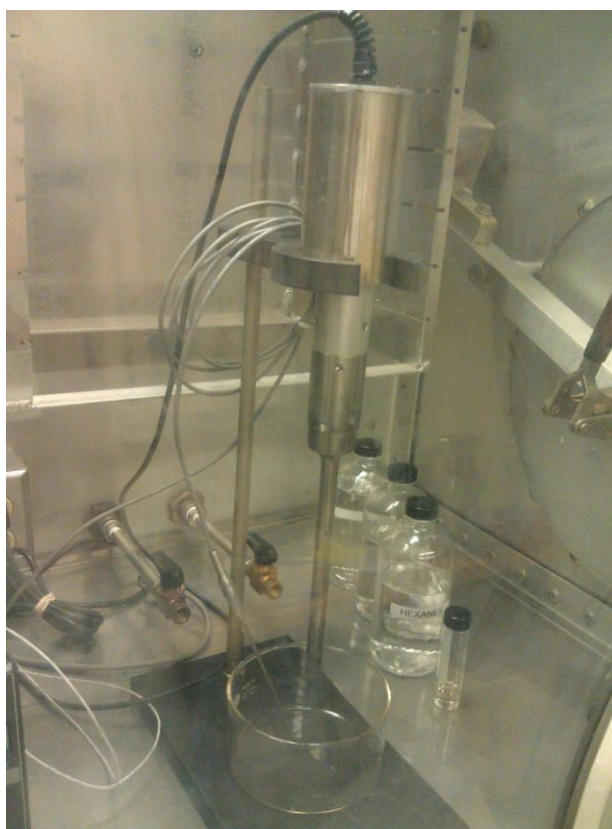
Figure 3.12 High-frequency ultrasonic probe located inside of a nitrogen glove box (an argon glove box appeared to cause shorting of the piezoelectric circuit due to arcing).
