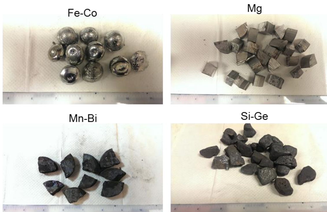
Figure A.5 Photographs of typical spark erosion charges measured with a ruler.
