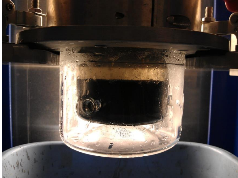
Figure A.2 Spark-eroded MnBi particle yield after 1 hour in a 4 inch ID glass pot. Rates of as high as 360 grams per hour have been achieved.
