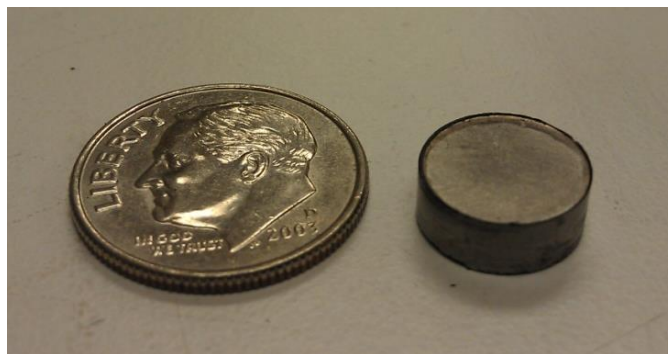
Figure 3.14 Bulk MnBi that has been compacted by RPS from spark-eroded MnBi powder compared to a U.S. dime. The nominal diameter of the compact is 3/8 inches.
