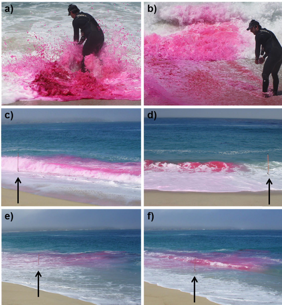
Fig. 3. Photos showing examples of (a) the initial dye slug release, (b) the well-mixed surf/swash zone shortly after the dye release, (c–d) turbulence and mixing of dye at the shoreline by breaking waves and alongshore advection of dye within the surfzone, and (e–f) run-down colliding with an incoming breaking wave resulting in the dye seeping offshore. Black arrows indicate locations of poles with dye sensors attached near the sea-bed in the surf zone, where (c–d) the intermittency of the dye observations is highlighted as the sensor is alternately submerged and not submerged.
