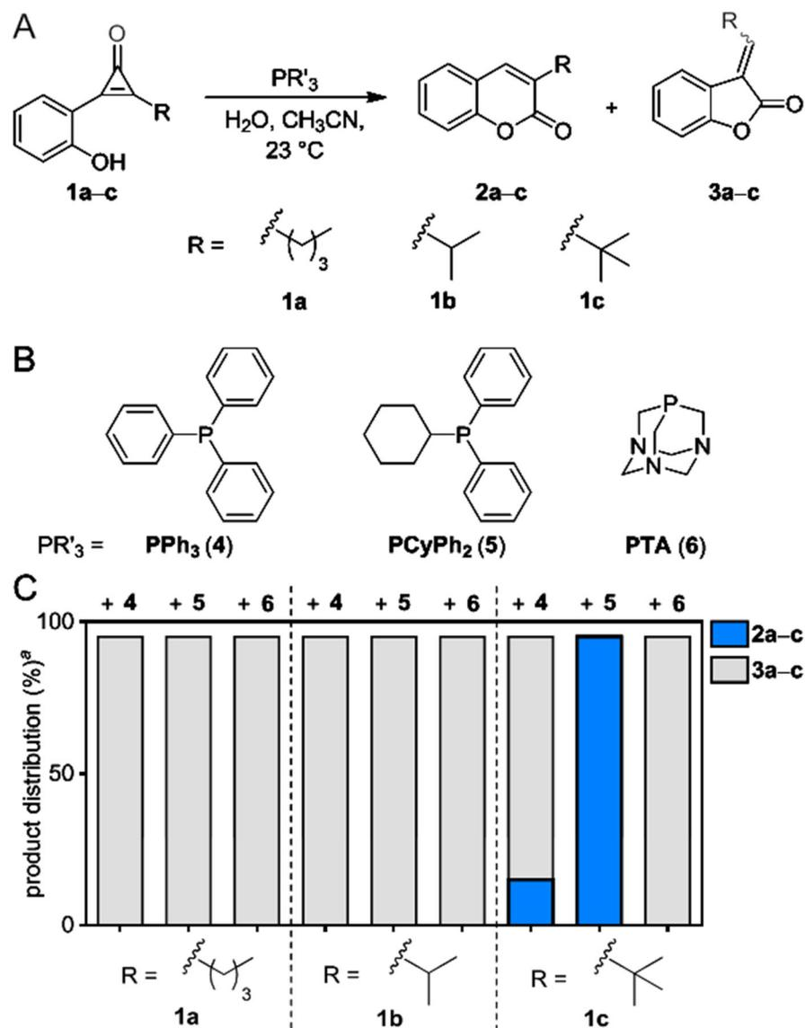
**Figure 3.** Distinct regioisomers are formed upon CpO treatment with various phosphines. (A) Phosphine activation of sterically modified CpOs can provide two cyclized adducts. (B) Structures of the phosphine probes examined. (C) Product distributions from treatment of CpO **1a-c** with phosphines **4-6**. <sup>a</sup>Yields measured by <sup>1</sup>H-NMR spectroscopy.
