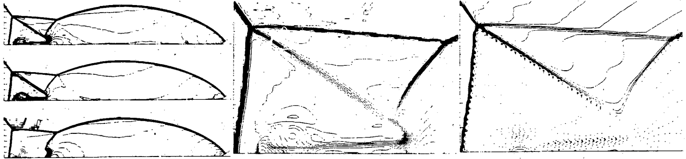
(a) \gamma = 1.40 ; (\rho, e, p) whole flowfield; (\rho, \tilde{M}) Mach stem region
