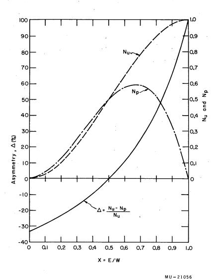
Fig. 1. Unpolarized (N<sub>u</sub>) and polarized (N<sub>p</sub>) positron spectra from the decay of 100% polarized muons at rest for  $\theta$  = 180 deg as given by the (V-A) theory. The asymmetry is  $\Delta$  = (N<sub>u</sub> - N<sub>p</sub>)/N<sub>u</sub>; the maximum positron energy is W = 52.86 Mev.
