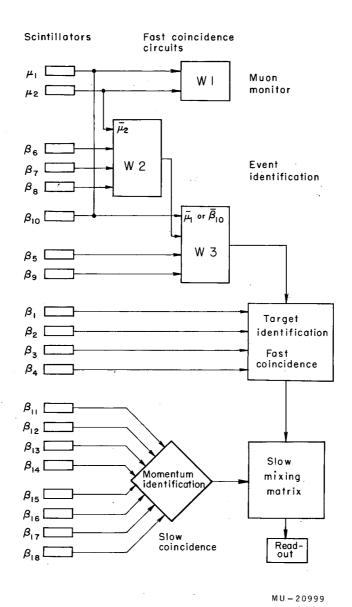
Fig. 9. Operational logic of the electronics used in this experiment.
