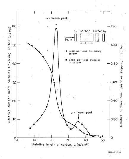
Fig. 3. Range curve of the meson beam. The absolute scale for the left abscissa is 10<sup>6</sup> per minute and that for the right abscissa is 10<sup>6</sup> per minute per 2.2 g/cm<sup>2</sup> carbon stopper.
