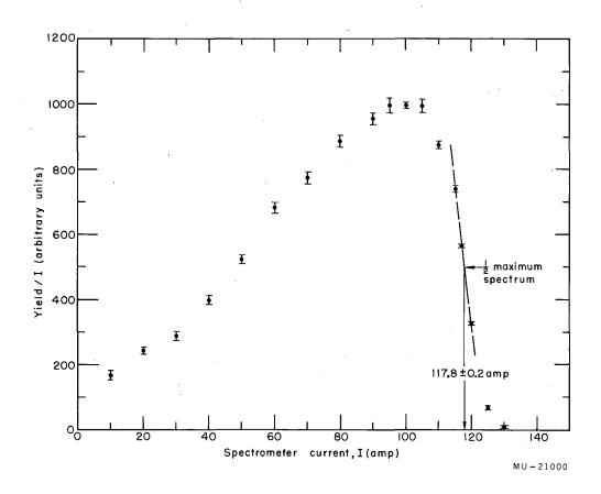
Fig. 11. Positron from unpolarized muons used to calibrate the spectrometer. The yield was divided by the current to remove the effect of the variation with current of the momentum band accepted by the spectrometer.
