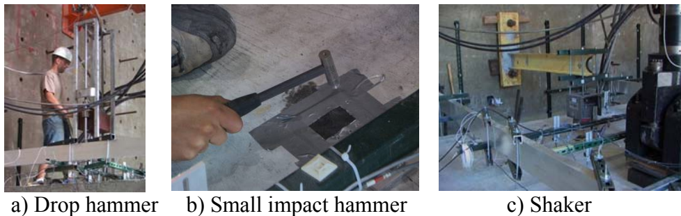
Figure 4.37 Forced excitation with three different excitation sources
