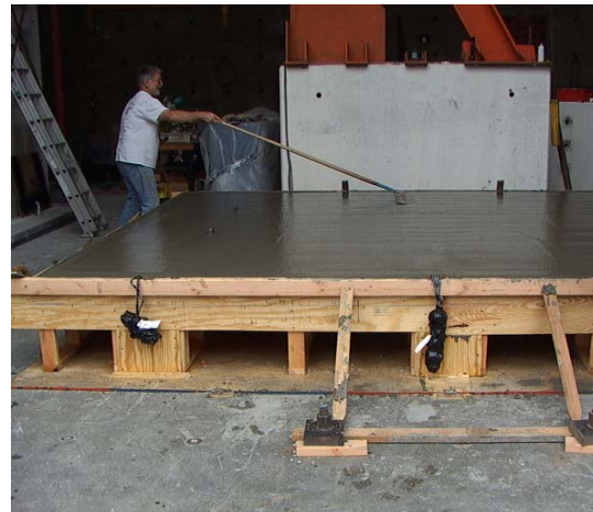
(b) Pouring of concrete and finishing of specimen surface
