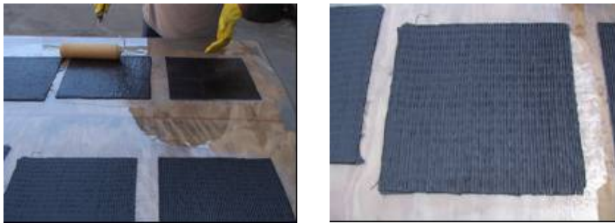
Figure 4.11 Manufacturing of composite panels for preliminary material tests
