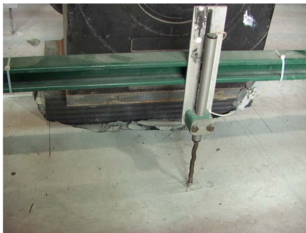
Figure 8.43 Crushing of concrete on slab top below load at 930 kN – Phase 3
