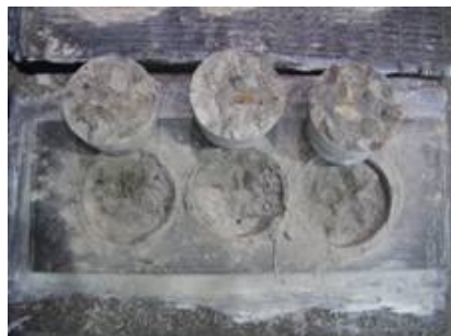
(b) Pull-off failures after tests
