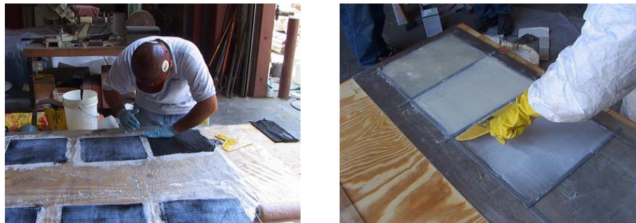
Figure 4.26 Manufacturing composite and resin test panels
