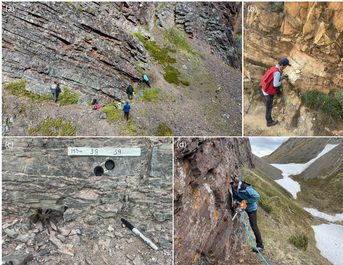
Figure 5.1: A paleomagnetic campaign. Samples consist in cylindrical pieces of rock (c) extracted from a given outcrop (a). Different layers are associated to different ages and sites. Pictures (b) and (d) despite Mathew Domeier measuring the orientation and drilling the new sample, respectively. Please notice that in all this chapter, samples correspond to rock samples, no statistical samples. Pictures courtesy of Leandro Gallo.
