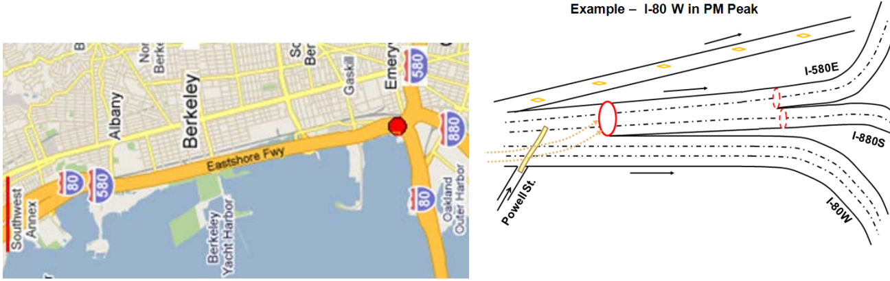
Figure 3.2. I-80 West PM peak section (L); Virtual lane drop and weaving at freeway diverge (R)
