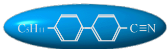
Figure 2.10: Anisotropic (rod-like) shape of a typical liquid crystal molecule. The molecule shown here is 4-cyano -4'- Pentylcyanobiphenyl, commonly known as 5CB, which exists in the nematic phase at room temperature.
