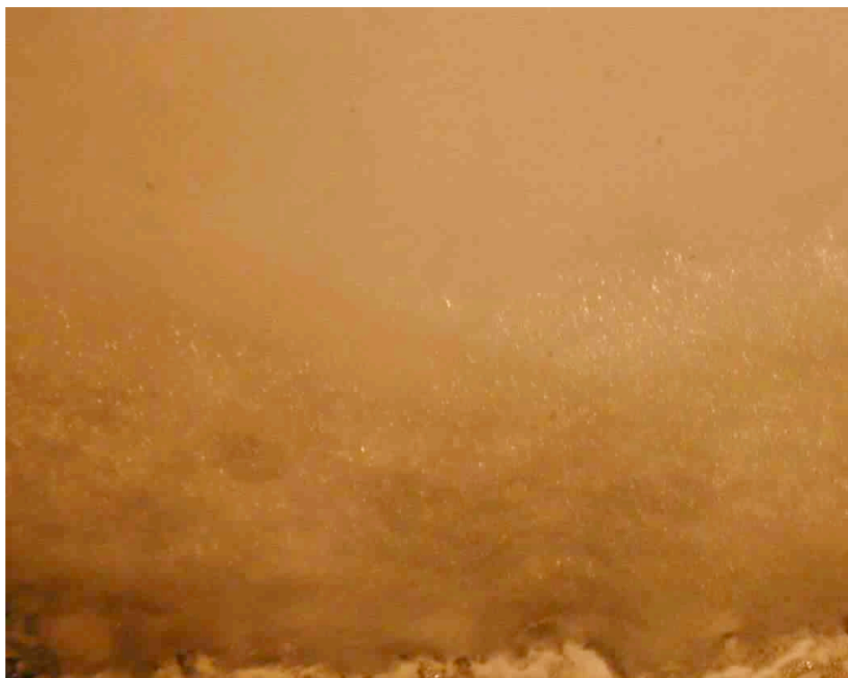
Photo 8 : K-Aluminosilicate phase transformation, snowy dull-like bubble structure, ~30X magnification.
