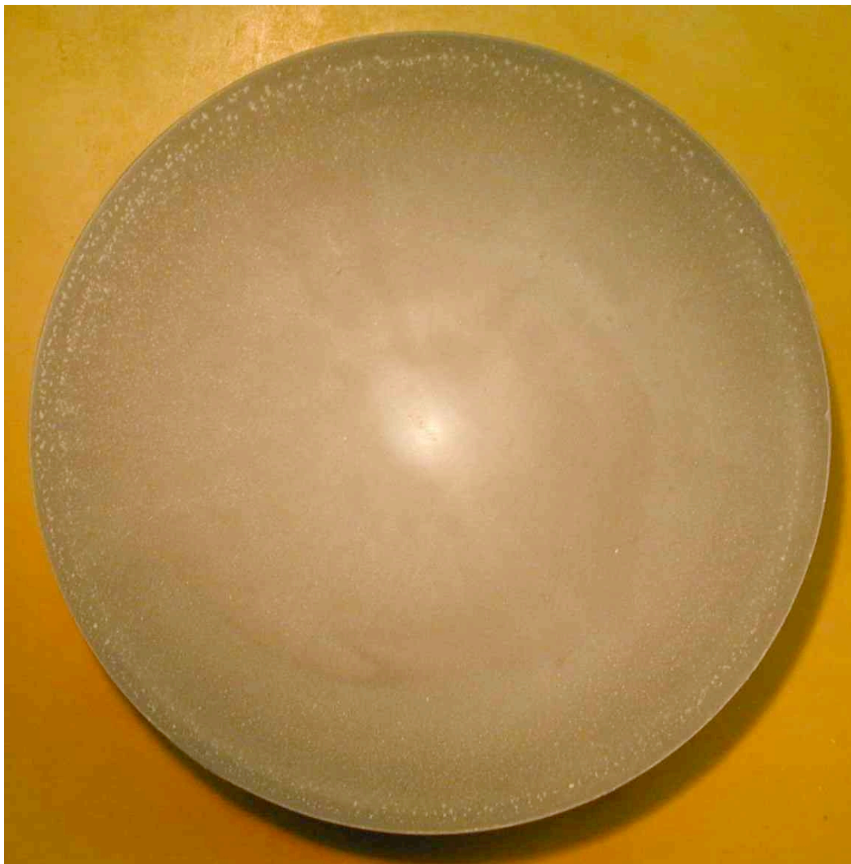
Photo 13 : After significant coating technique improvements to fabricate 10cm diameter, 0.5 mm thick K-alumino-silicate coating on porous tungsten substrates for HCX source.
