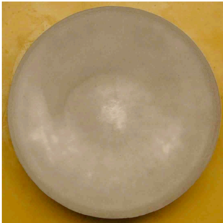
Photo 10 : K-Aluminosilicate coating thickness vs. phase structure on 10cm diameter substrate.
