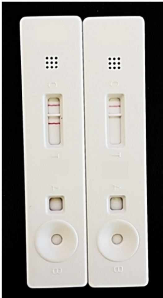
Fig. 2. LFA test. Shown are results of the LFA run with positive (left) and negative (right) control sera.
