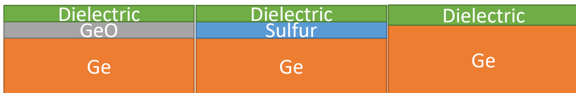
Figure 4.2 – (left) GeO passivation, (middle) sulfur passivation, and (right) dielectric passivation.
