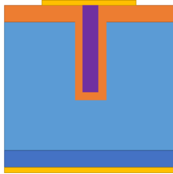
Figure 3.35 – Deep pit photodiode structure with the center conductor replaced with a scintillator.
