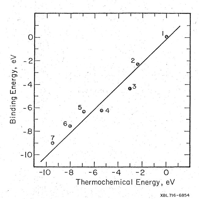
Fig. 1 Plot of boron <u>ls</u> binding energies <u>vs</u> thermodynamically estimated binding energies.
