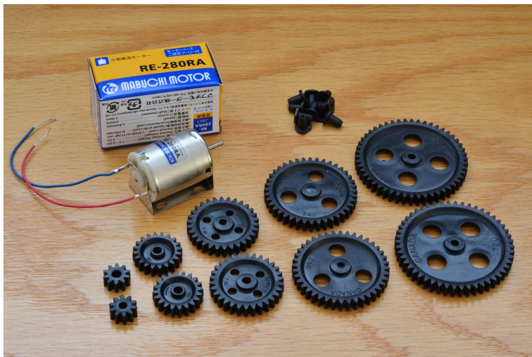
Figure 3: The Mabuchi RE-280RA permanent magnet DC motor and plastic spur gear sets (two each of 10, 20, 30, 40, and 50 tooth sizes) with inserts.
