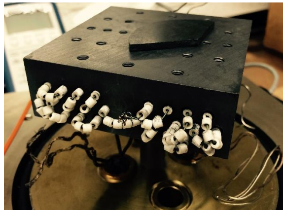
Fig. 2.2 Photo of the graphite heating platform
