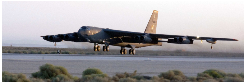
Figure 3.2: A B-52 Stratofortress takes off from Runway 22 during a Fischer-Tropsch test flight from Edwards Air Force Base, Calif., on Sept. 19, 2006. During the flight, two of the aircraft’s eight engines ran on the natural gas-based Fischer-Tropsch fuel blend. The bombers are from the 5th Bomb Wing at Minot Air Force Base, N.D. (U.S. Air Force photo/Chad Bellay).
