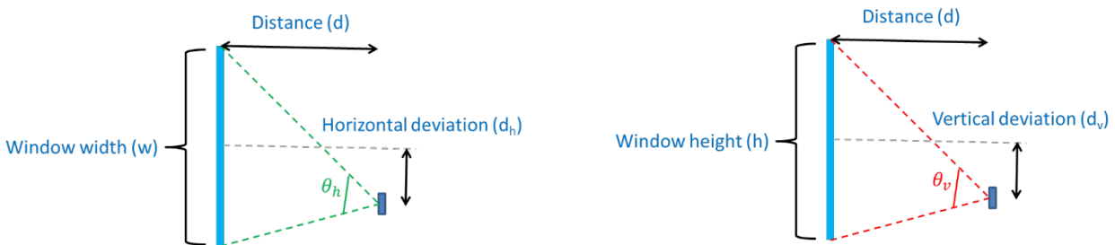
Figure 3. The calculation of thermostat view factor. Left: plan of view factor seen by object; Right: elevation of view factor seen by object.
