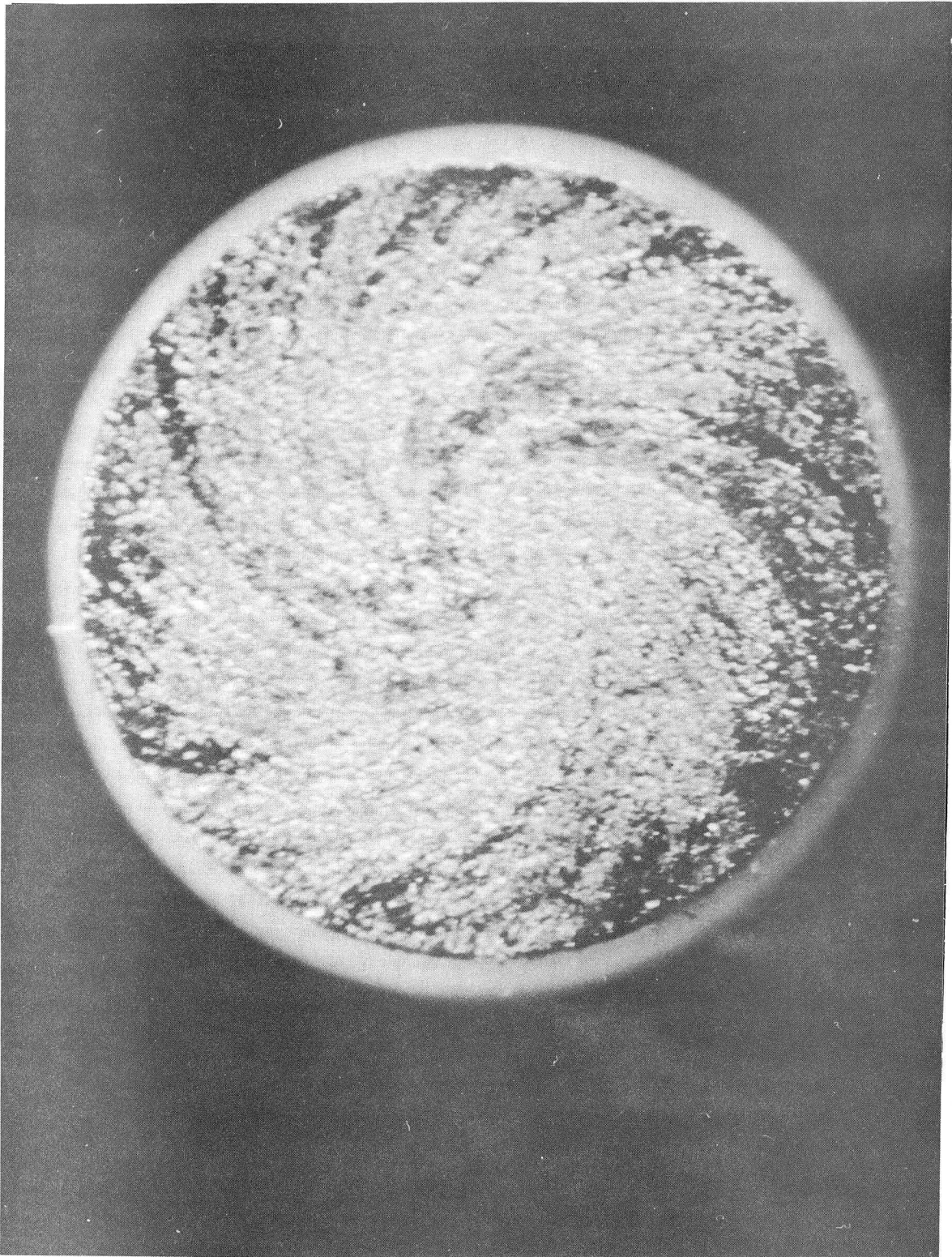
Fig. IV-1. Mg deposit on a Pt rotating-disk electrode. Electrolyte: 0.5M \text{MgCl}_2 and 1.0 M \text{NaBH}_4 in PC. i = 1.0 \text{ mA/cm}^2 . Rotation speed \omega = 3600 \text{ rpm} .
