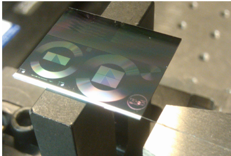
Figure 114: Picture of fabricate 2-layer core. Spiral 2 and Spiral 3 are shown here.
