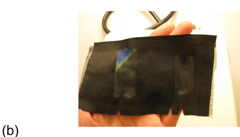
**Figure 32** (a) Color changes that occur on heating a swatch of silk painted with two thermochromic liquid crystal paints. (b) The color change reverses as the silk cools back to room temperature, as shown here by blocking the source of heat.
