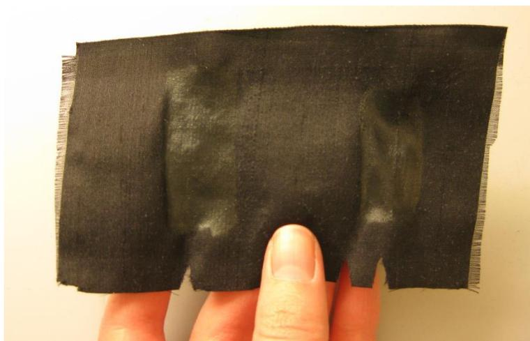
**Figure 31** A piece of silk fabric, with one thermochromic liquid crystal paint on the left (active in the 95-104°F range), and another on the right (active in the 104-113°F range).
